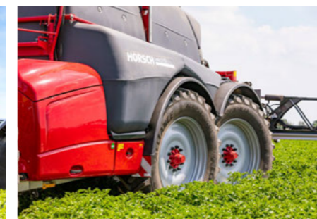
High manoeuvrability and stability with a clearance of up to 90 cm
