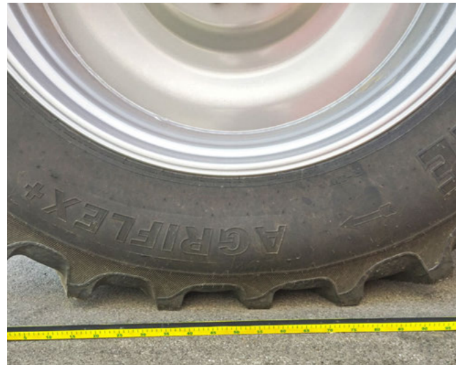
ATP Control – smooth running with a tyre pressure of 2.3 bar
