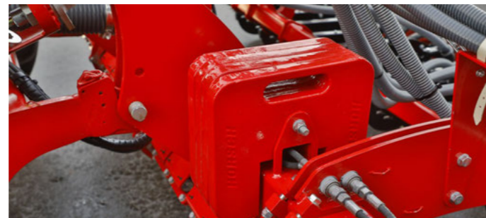
Additional weights for the NT CoulterBar
