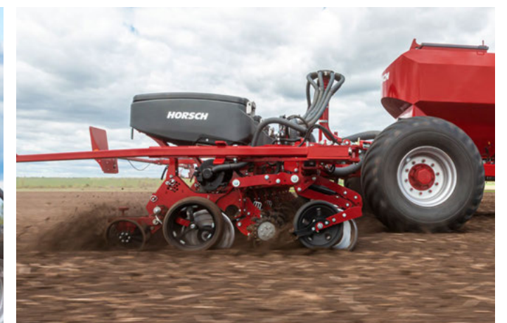
Single disc fertiliser coulter, spokes depth control wheel and finger wheel ideal for black earth soil soils
