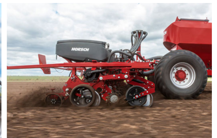
Single disc fertiliser coulter, spokes depth control wheel, and finger roller ideal for brown soil
