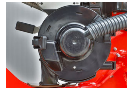
Easily accessible metering units with different metering discs depending on the type of crop
