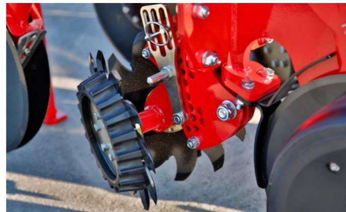
Optional trash wheels, floating with depth control
