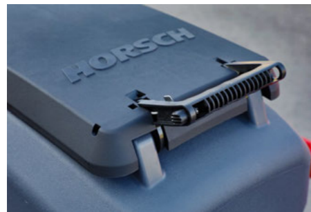
Lock row container
