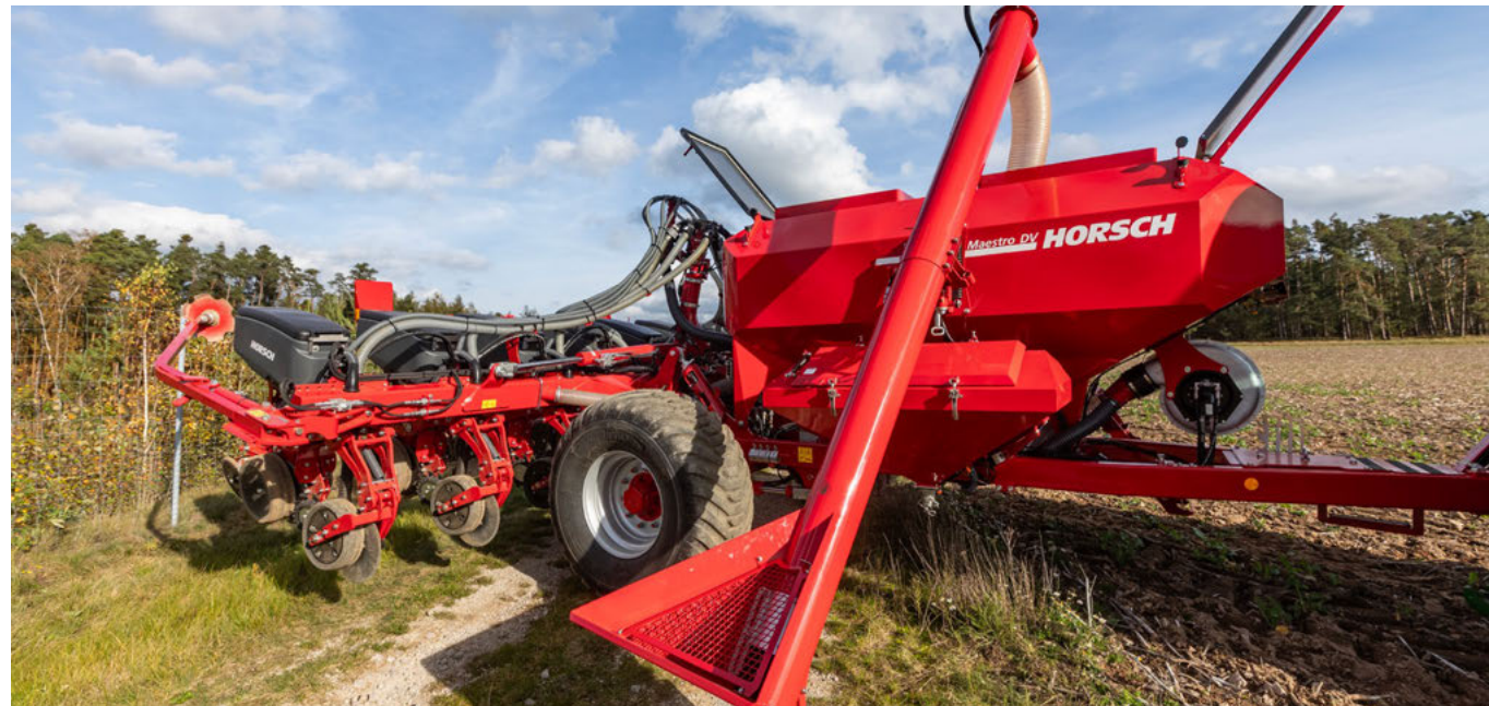
The filling auger can be used for both fertiliser hoppers of the Maestro DV
