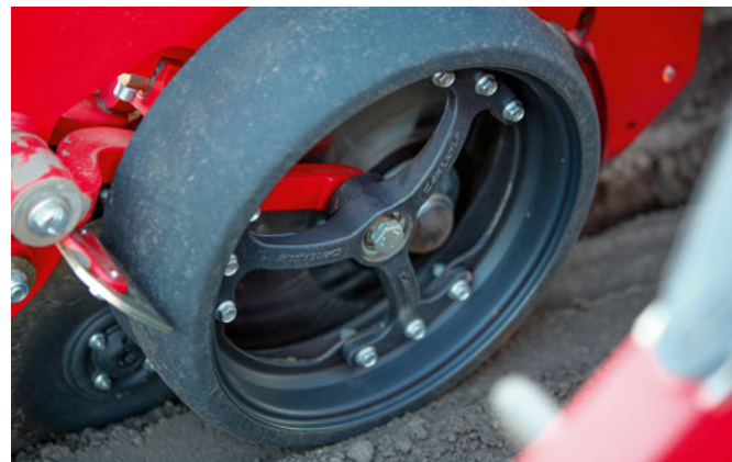
Spokes depth control wheel: better self-cleaning, thus ideal on black earth soils
