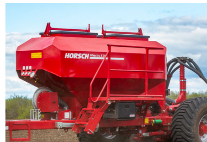
Double hopper system with a capacity of 3 500 l
