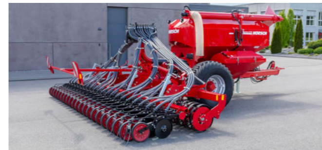
6 TD CoulterBar for offset row seeding at Maestro DV
