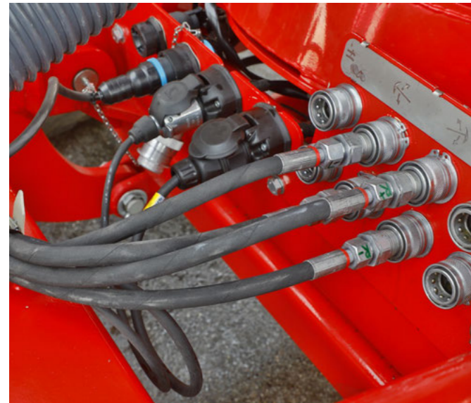
Clear cut-off point for hydraulics and pneumatics
