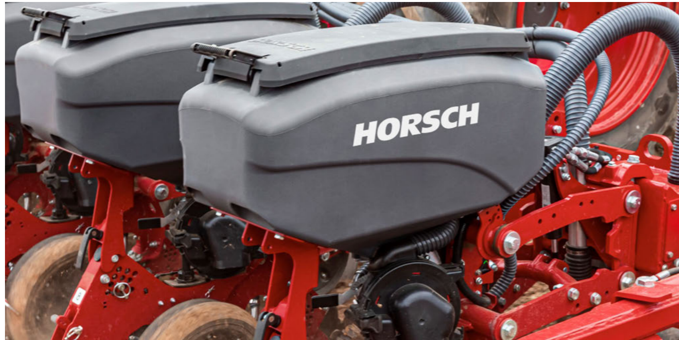
Row unit hopper with a capacity of 70 l
