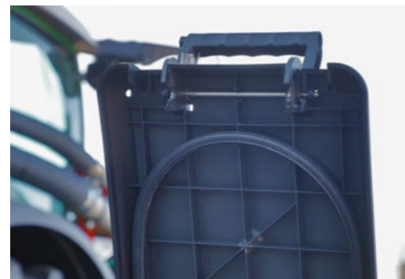
Cover seal row unit hopper
