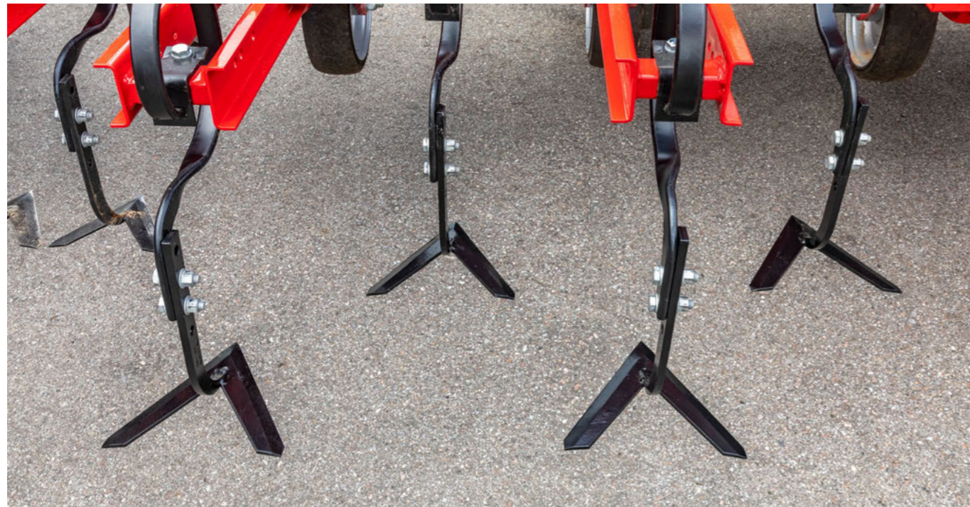
Parallelogram equipment for 25 cm row spacing
