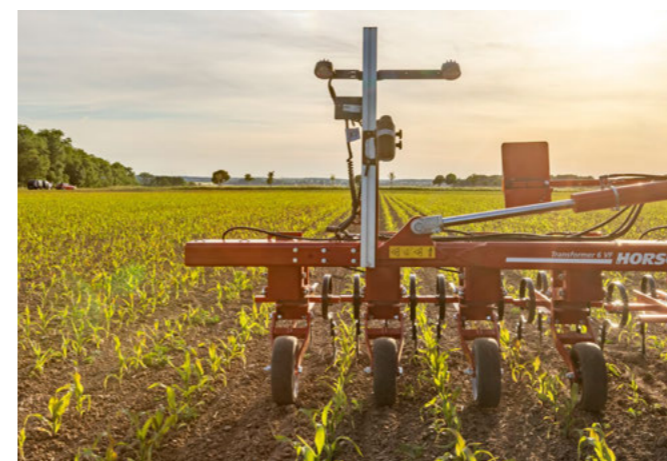
Runs along the plant row with utmost precision due to the optional camera Culticam
