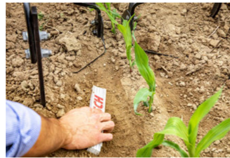
Angle knives cut precisely along the plant row
