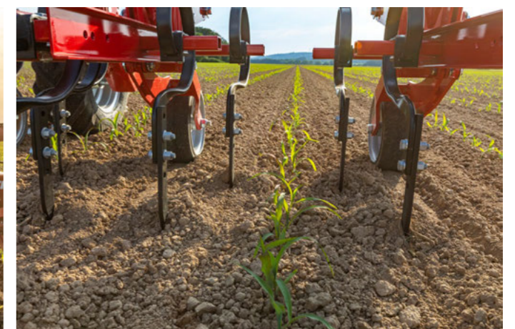
Reliable and precise hoeing along the plant row in different growth stages
