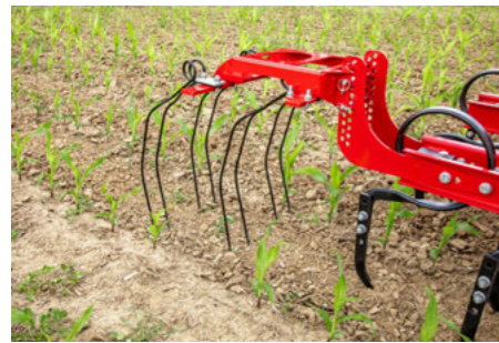
Following harrow removes soil from cut weeds
