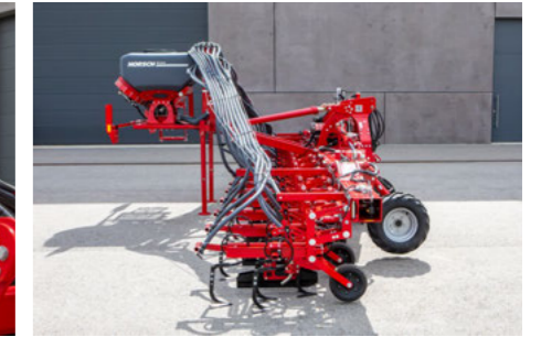
Transformer 9 VF equipped with MiniDrill
