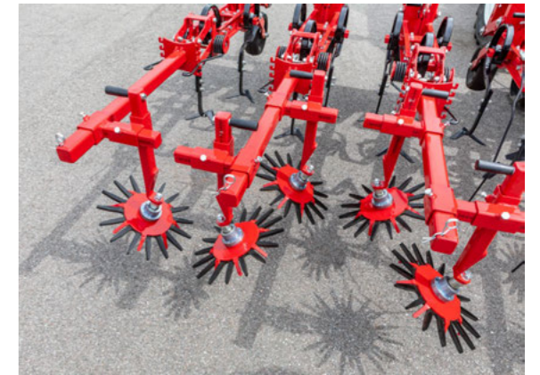
The finger hoe allows for working precisely at or in the plant row, e.g. for maize.
