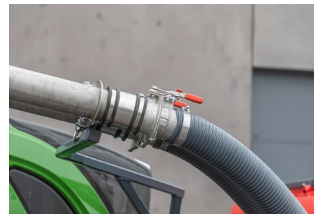
Quick couplings help a fast coupling and decoupling between front hopper, tractor console and implement
