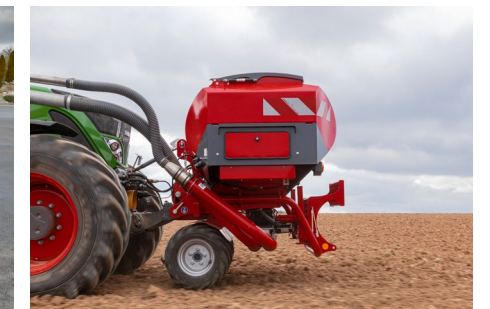
The tyre packer allows for pressing and crushing clods
