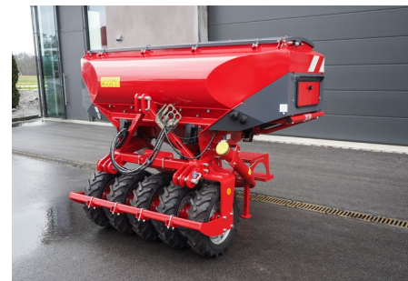
The tyre packer guarantees even and consolidated conditions
