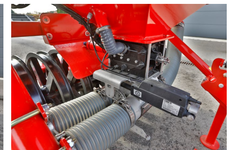
Partner 1600 FT with electric half-width shut-off
