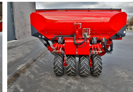
1.30 m wide contact area over 4 tyres and additional weights
