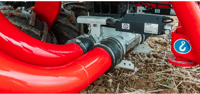
Electric half-width shut-off – switching the half-width on and off easily via a button in the terminal
