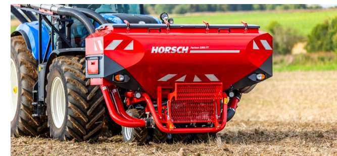
Partner 2000 FT with 60:40 partition allows for applying seed and fertiliser, 2 x seed or two different fertilisers
