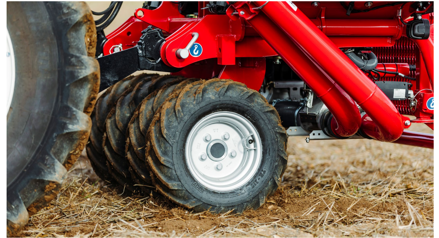
In the field, the tyre packer allows for an optimum soil presentation
