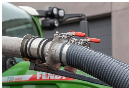
Easy handling of the pneumatic tubing without tools
