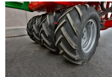
20° passively controlled tyre packer
