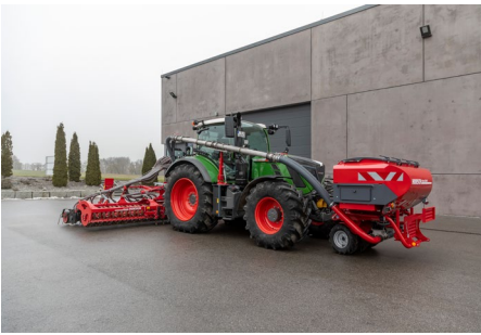
Horizontal tubing attachment ensures minimum visibility restrictions
