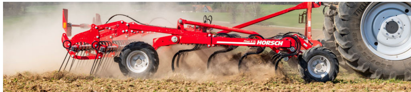
Four depth control wheels which are mounted at the packer Packer can be replaced by rear depth control wheels
