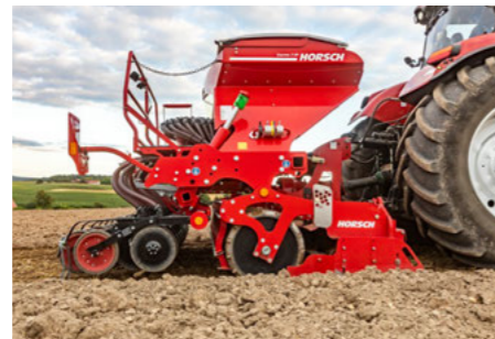
When using the power harrow solo on the headlands, the seed bar can be lifted hydraulically.
