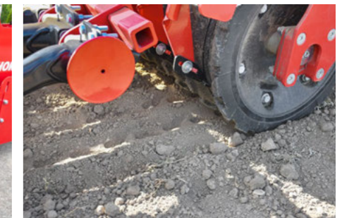
FarmFlex packer Strip consolidation reduces encrusting
