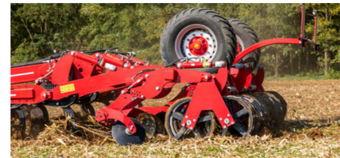
Wide selection of packers due to swivel chassis
