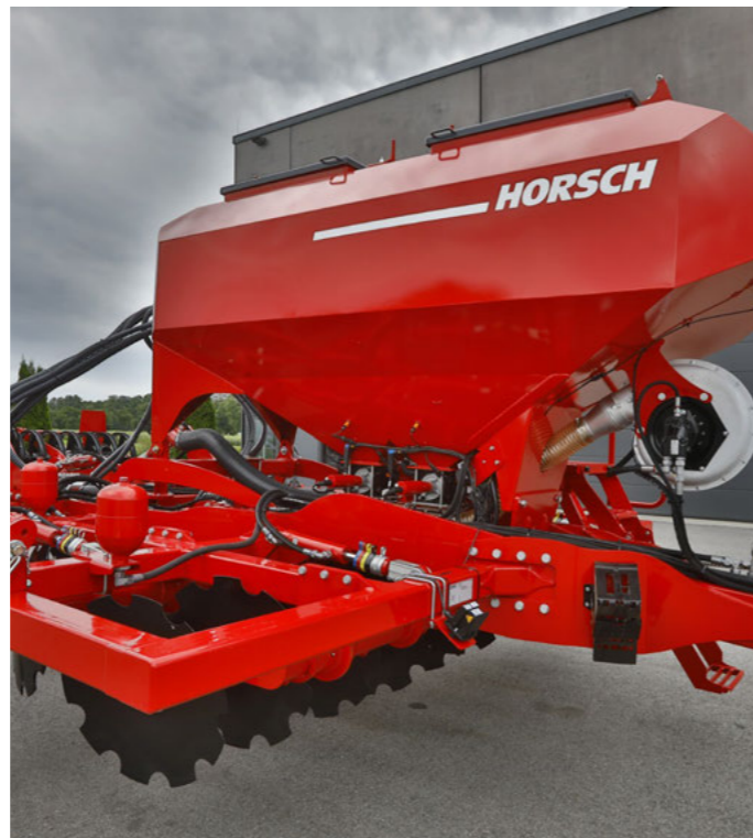
FertiProf with a hopper capacity of 2 800 l for direct fertilisation in one pass
