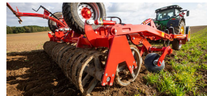
Double RollPack packer with swivel transport wheels
