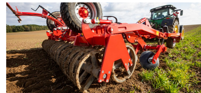
Double RollPack packer with swivel transport wheels
