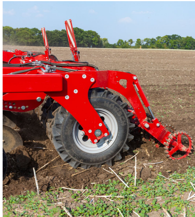
TopRing packer for an efficient consolidation between the tyres
