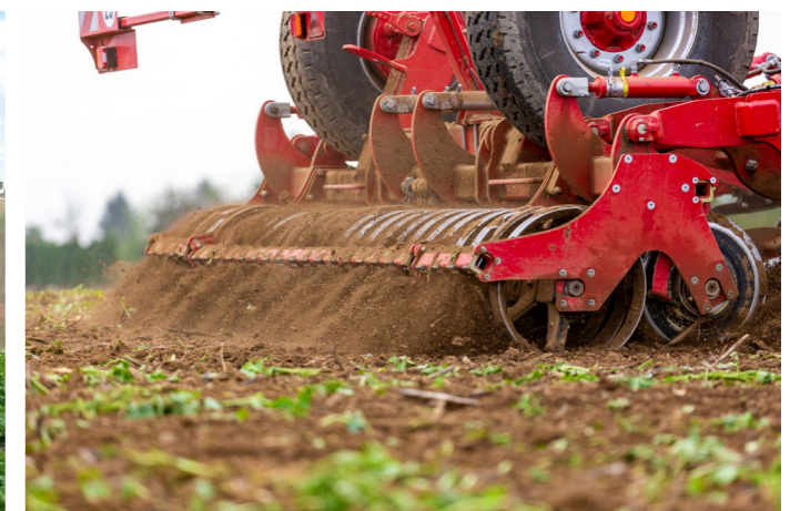
High fine soil production due to SteelFlex packer
