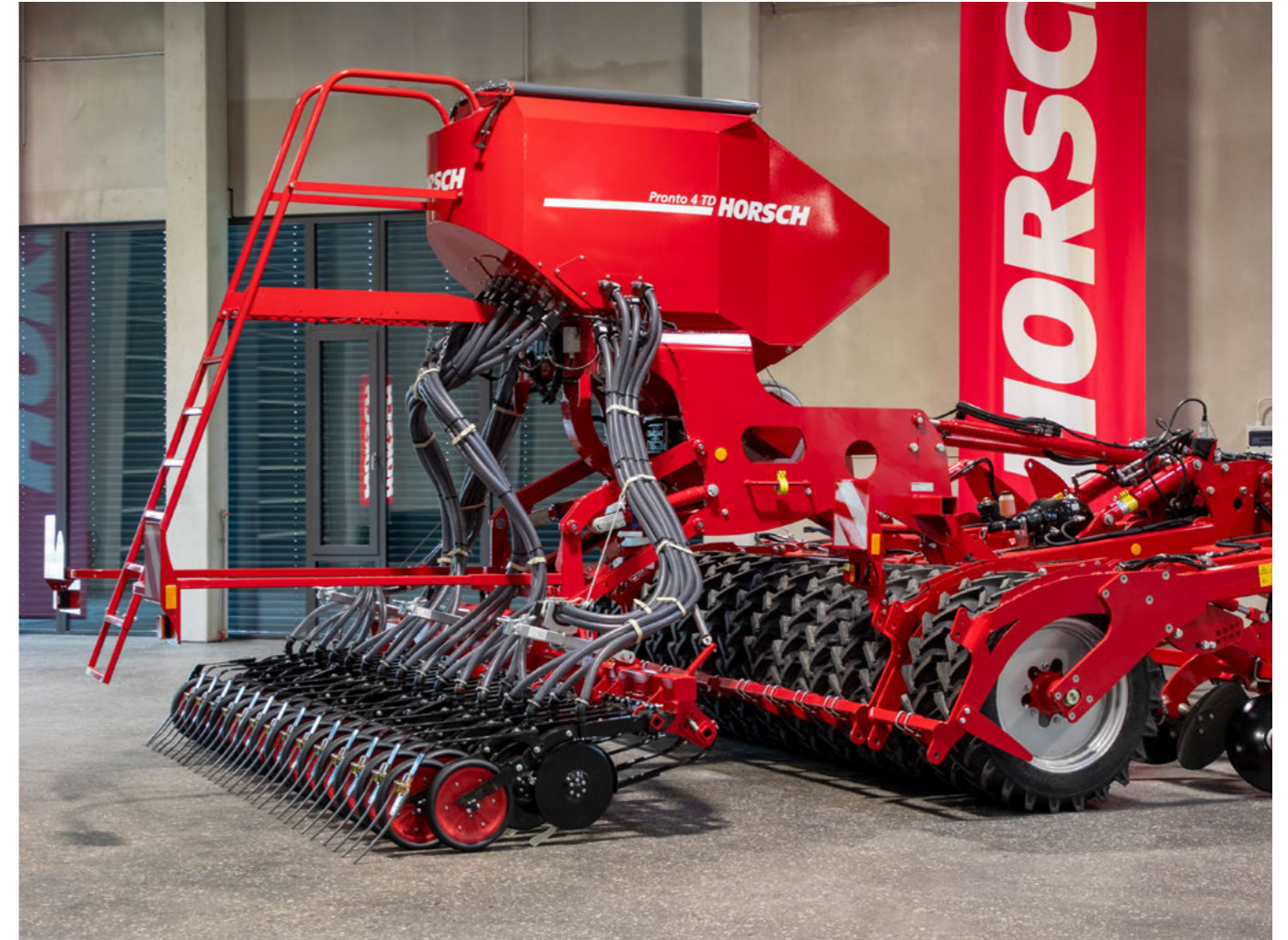
Pronto TD to combine primary soil cultivation and sowing
