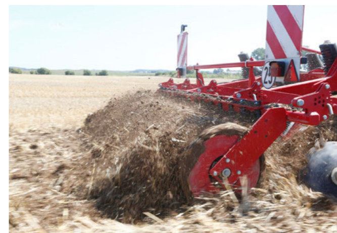
Packers produce much fine soil for optimum germination conditions
