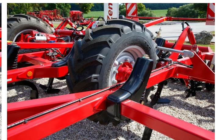
Large tyres for road transport and depth control when driving without a packer
