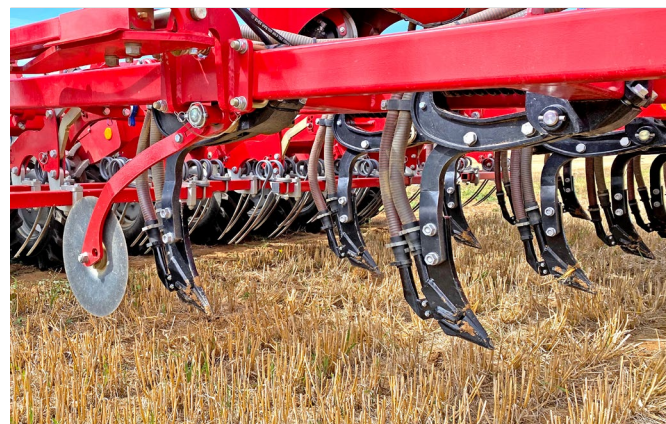
Minimum opening of the soil with the ThinEdge coulter
