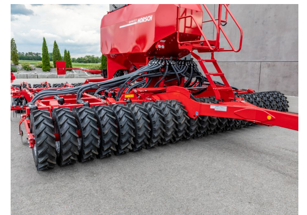
Even consolidation due to packer
