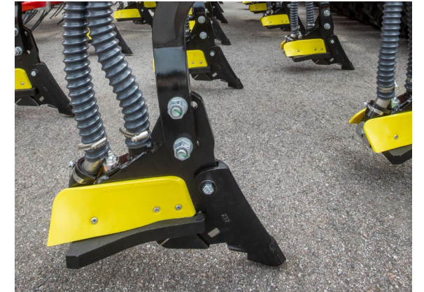
Fertiliser and seed placement with the Duett coulter
