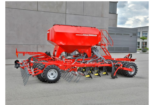
The 2-row harrow ensures an optimum covering of the grain
