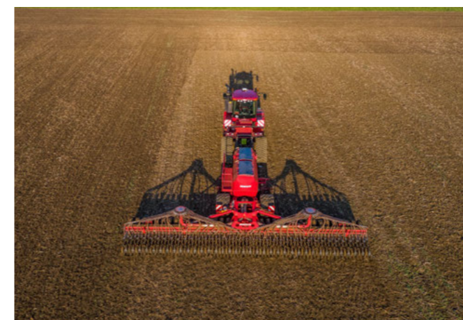
Safe maintenance of the set placement depth across the whole working width due to hydraulic weight transfer of the seed wagon weight to the coulter wings
