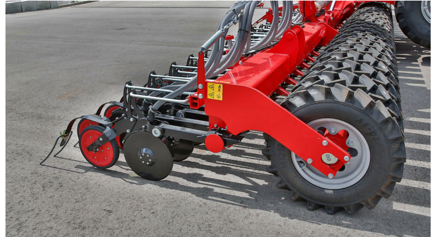
PowerDisc seed coulters – parallel-disc controlled double disc coulters
