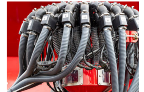
RowControl distribution tower
