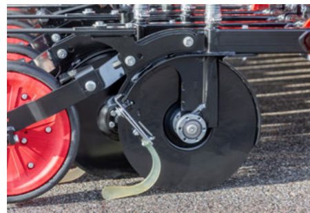
Fall tube position in front of the mounting and moving inside scraper prevent blockage of the coulters in wet sowing conditions
