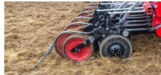
Coulters pressure up to 200 kg is possible
