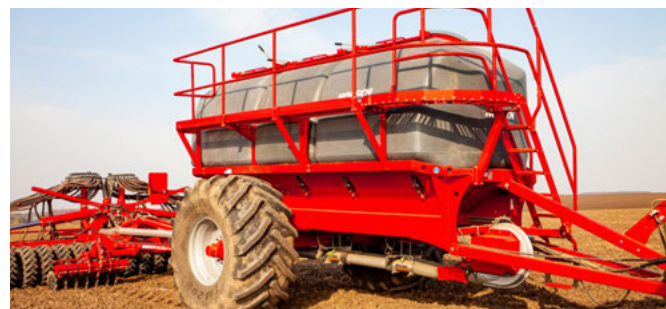
Double hopper with a partition of 8 500 l : 8 500 l or triple tank with a partition of 4 000 l : 6 500 l : 6 500 l
