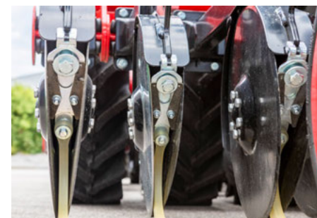
The movable scraper ensures a high self-cleaning effect in wet conditions
