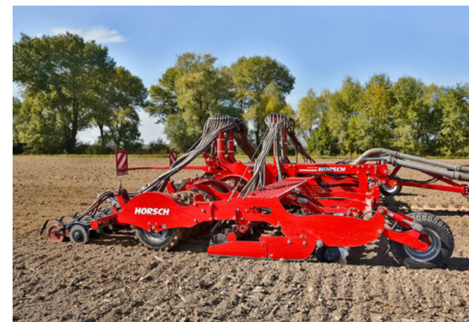
TurboDisc seed coulters for precise seed placement and high coulters pressures
