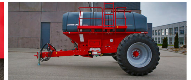
Option for two other components like solid fertiliser and seed in the second and third hopper
