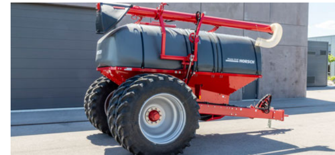
Hydraulic filling auger for an autarkic filling
