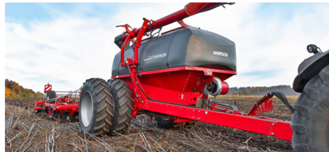
Double hopper a partition of 6 000 l : 6 000 l or triple tank with a partition of 4 000 l : 2 000 l : 6 000 l
