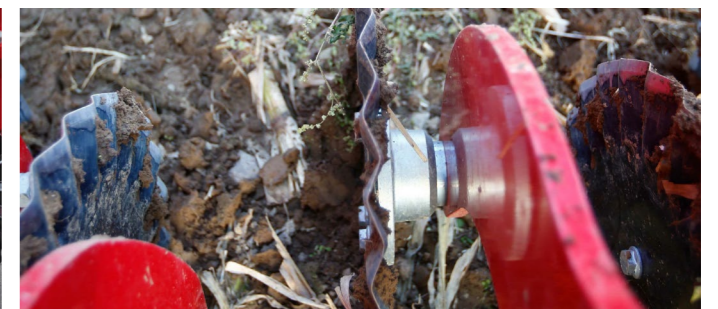
Removal of harvest residues and plant material from the seed strip
