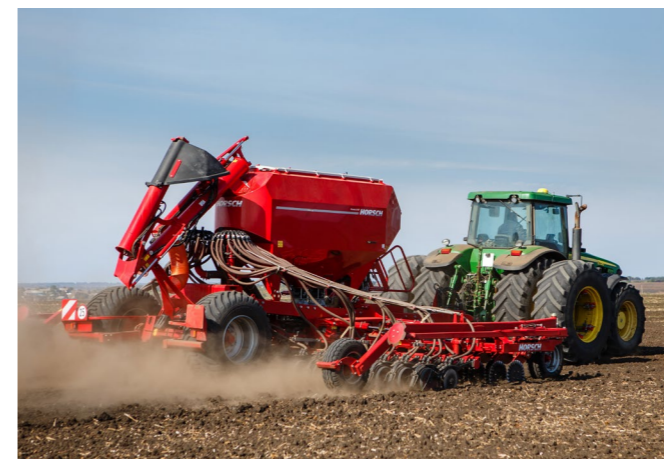
Hydraulic filling auger with an output of up to 800 kg/min
