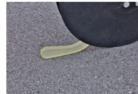
The HORSCH Uniformer ensures a precise fixing of the seed
