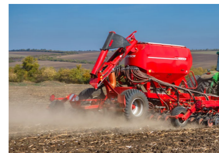
Easy filling due to hydraulic filling auger
