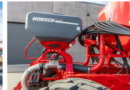
400 l rapeseed seed in the MiniDrill allows for filling the other hoppers with mineral fertiliser.
