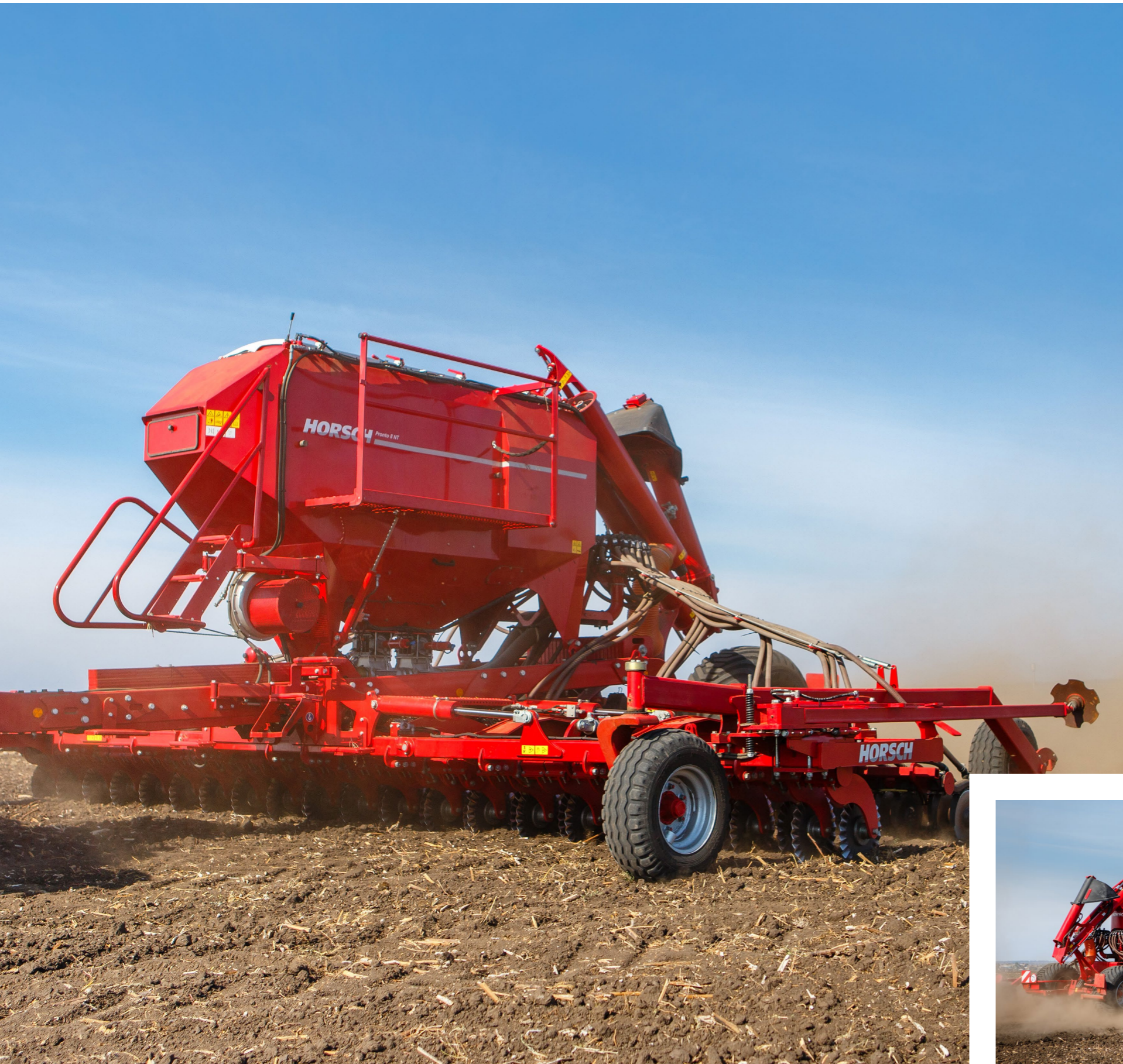
Hydraulic filling auger with an output of up to 800 kg/min
