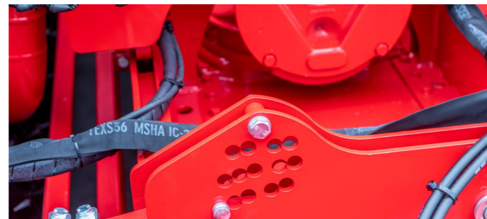
Working depth adjustment of the Kredo power harrow
