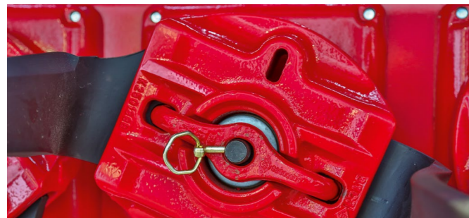
Tines can be changed without any tools
