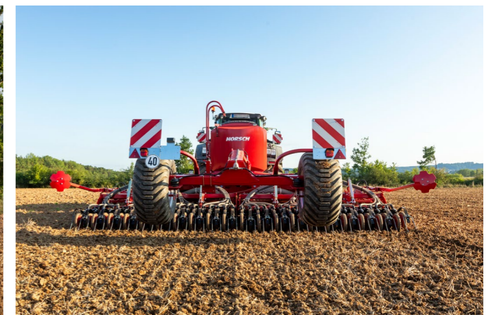
Integrated pivoted frame for more precision – every machine half can independently adapt its angle to the terrain
