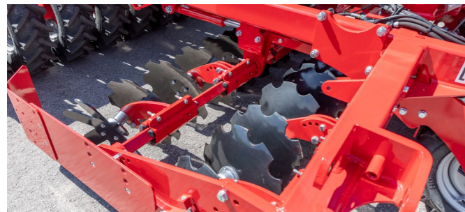
DiscSystem Pronto DC with attachment frame for track eradicator discs
