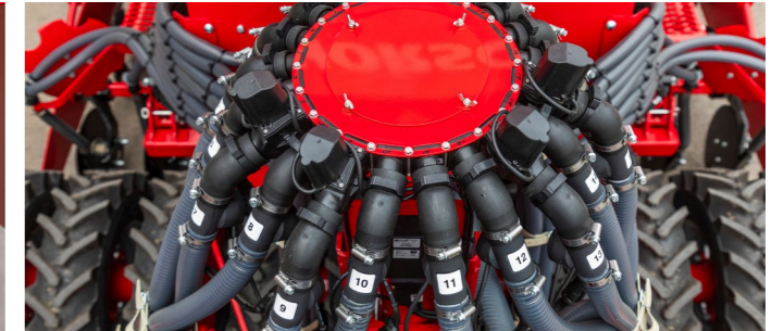
Monitoring of the pneumatic flow at the distribution tower
