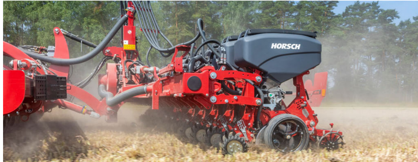
With seed wagon attachment, a coulter pressure of up to 350 kg is available
