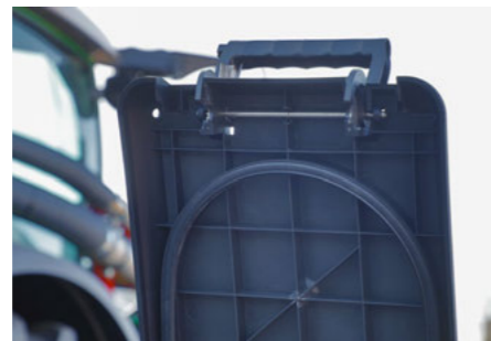
Cover seal row unit hopper
