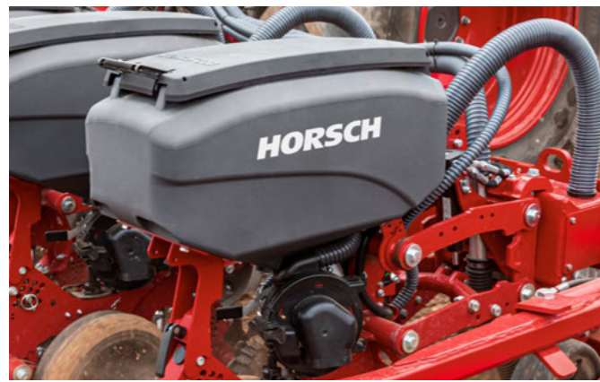
Row unit hopper with a capacity of 70 l
