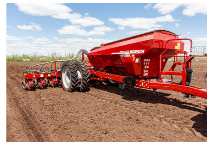
Fertiliser hopper 3 000 l and central seed hopper with a capacity of 800 l
