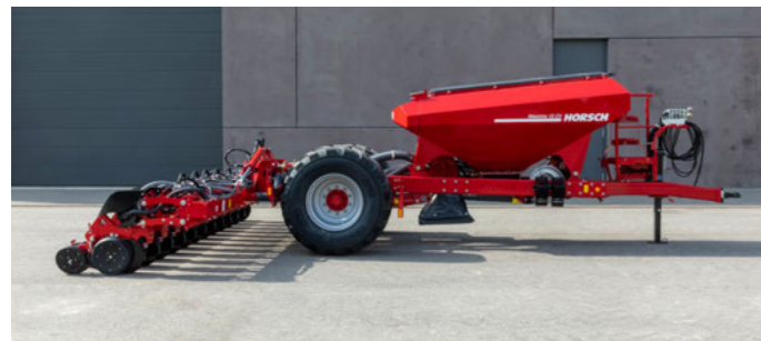
Seed-Only version with a seed capacity of 3 000 l
