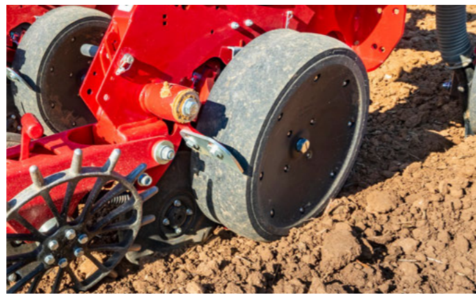
Standard depth control wheel for normal soils
