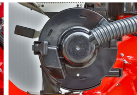
Easily accessible AirVac metering device
