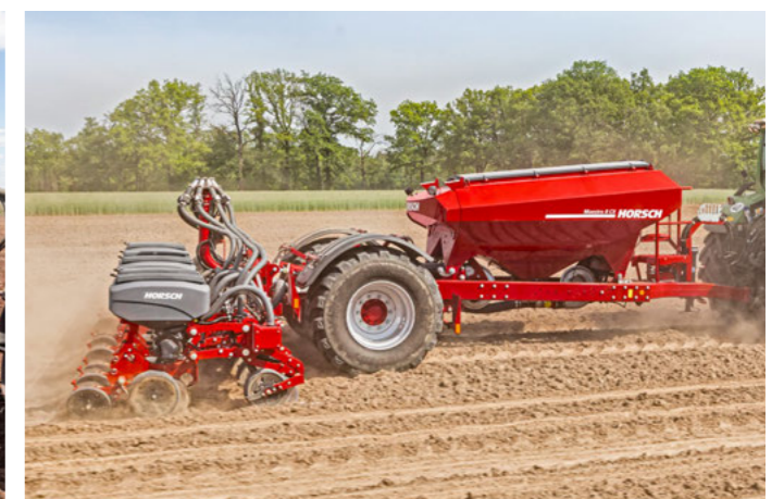
Maestro 8 CX with row unit hopper for sowing maize
