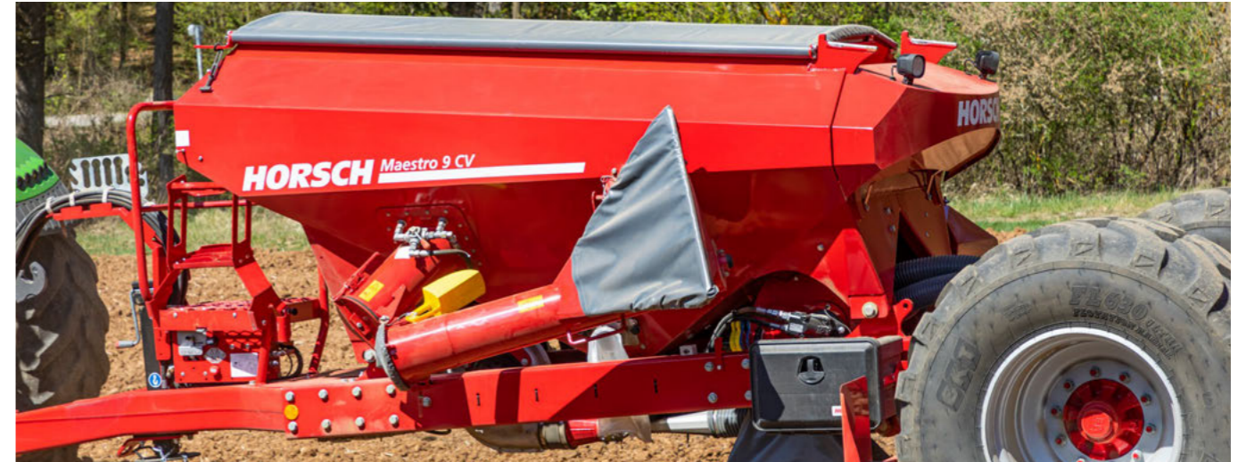
Folded, hydraulic filling auger fertiliser tank
