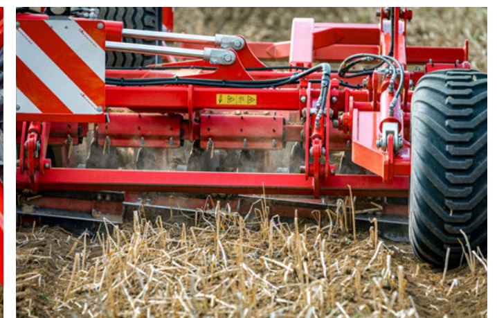
Knife roller for additional crushing
