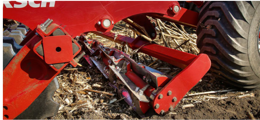
Knife roller for Joker 5-8 RT Hydraulically pre-stressed knife roller for additional crushing effect
