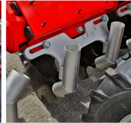
Liquid manure outlets made of stainless steel for long service life
