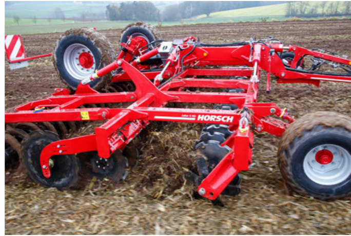
Large disc spacing for maximum clearance in the machine
