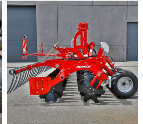
Liquid manure version without packer, with harrow to guarantee a low susceptibility to clogging
