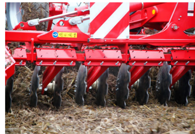
Width of disc bearing on the frame for exact control of the discs in the soil
