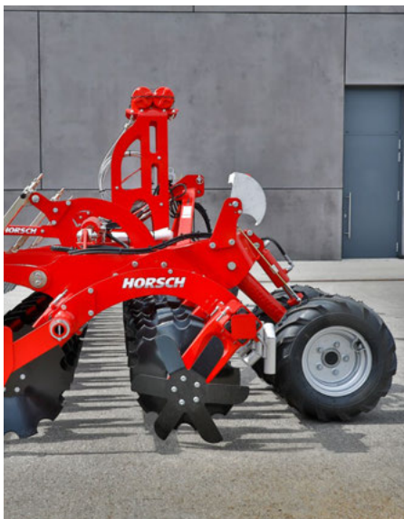
Liquid manure version without packer, with harrow to guarantee a low susceptibility to clogging
