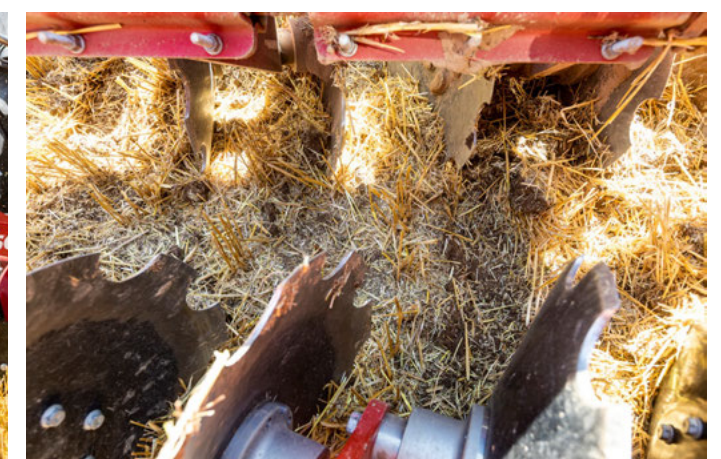
Discs are arranged in pairs for maximum clearance
