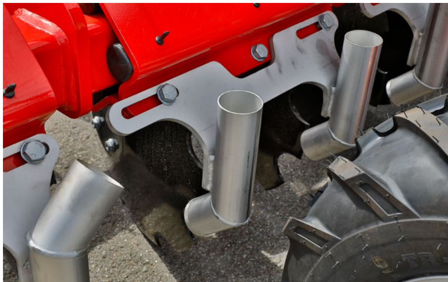
Liquid manure outlets made of stainless steel for long service life
