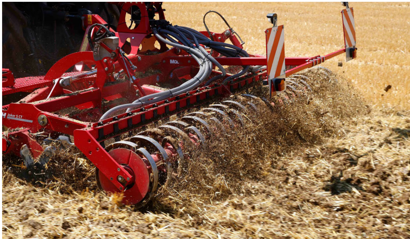
Option: MiniDrill for sowing catch or cover crops
