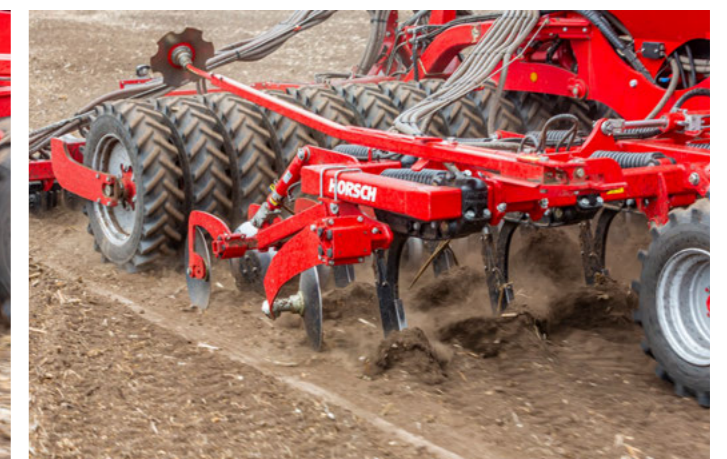
LD points take moisture into the seed horizon
