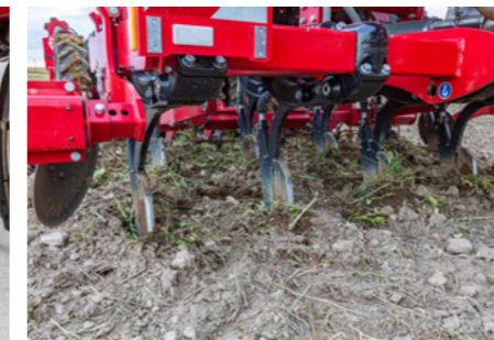
ULD point opens the soil and places fertiliser
