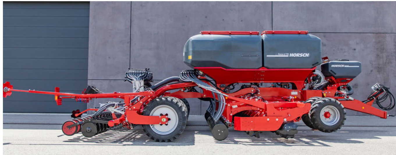
Large tyre packer for deep consolidation
