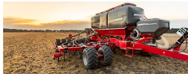
MiniDrill G&F – application of a third component
