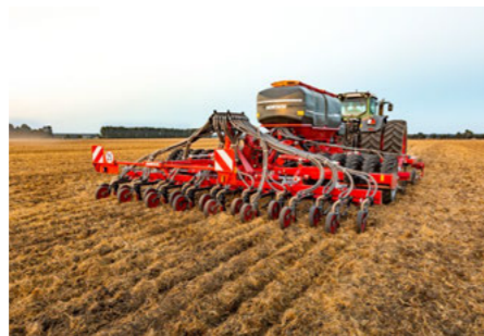
TurboEdge seed coulter for sowing in soils with a lot of straw
