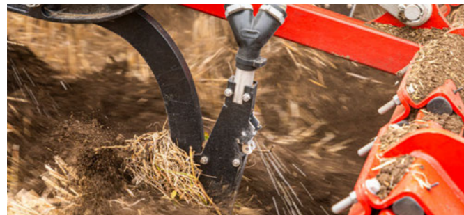
LD point /LD Plus point – fertiliser application in the upper horizon
