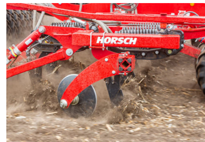
LD point ensures a good mixing of the soil
