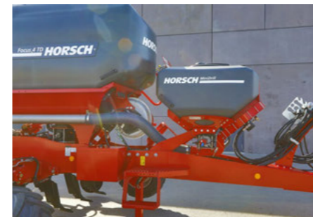
MiniDrill PPF – third component can be applied to another horizon
