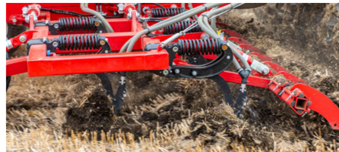
LD point /LD Plus point – mixing of the loosened area
