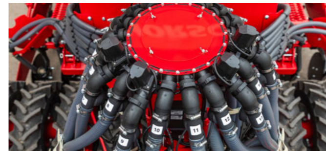
Monitoring of the pneumatic flow at the distribution tower
