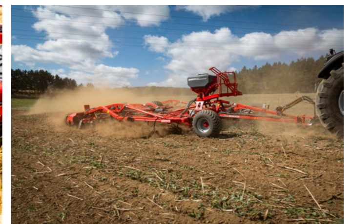
A full-surface cut is also possible with 20 cm wing points.
