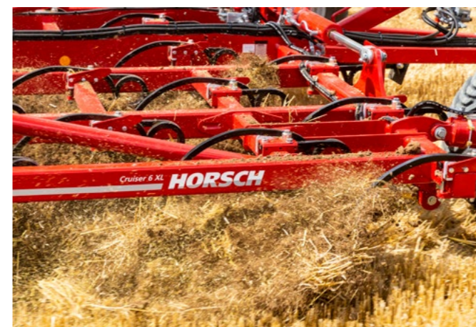
HORSCH spring tines with 150 kg pre-tension force
