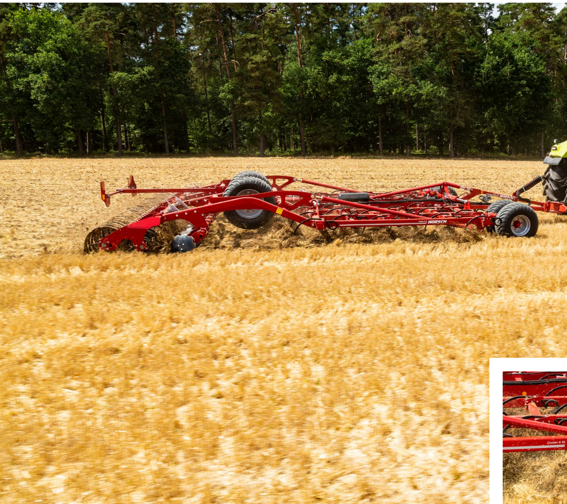
HORSCH spring tines with 150 kg pre-tension force
