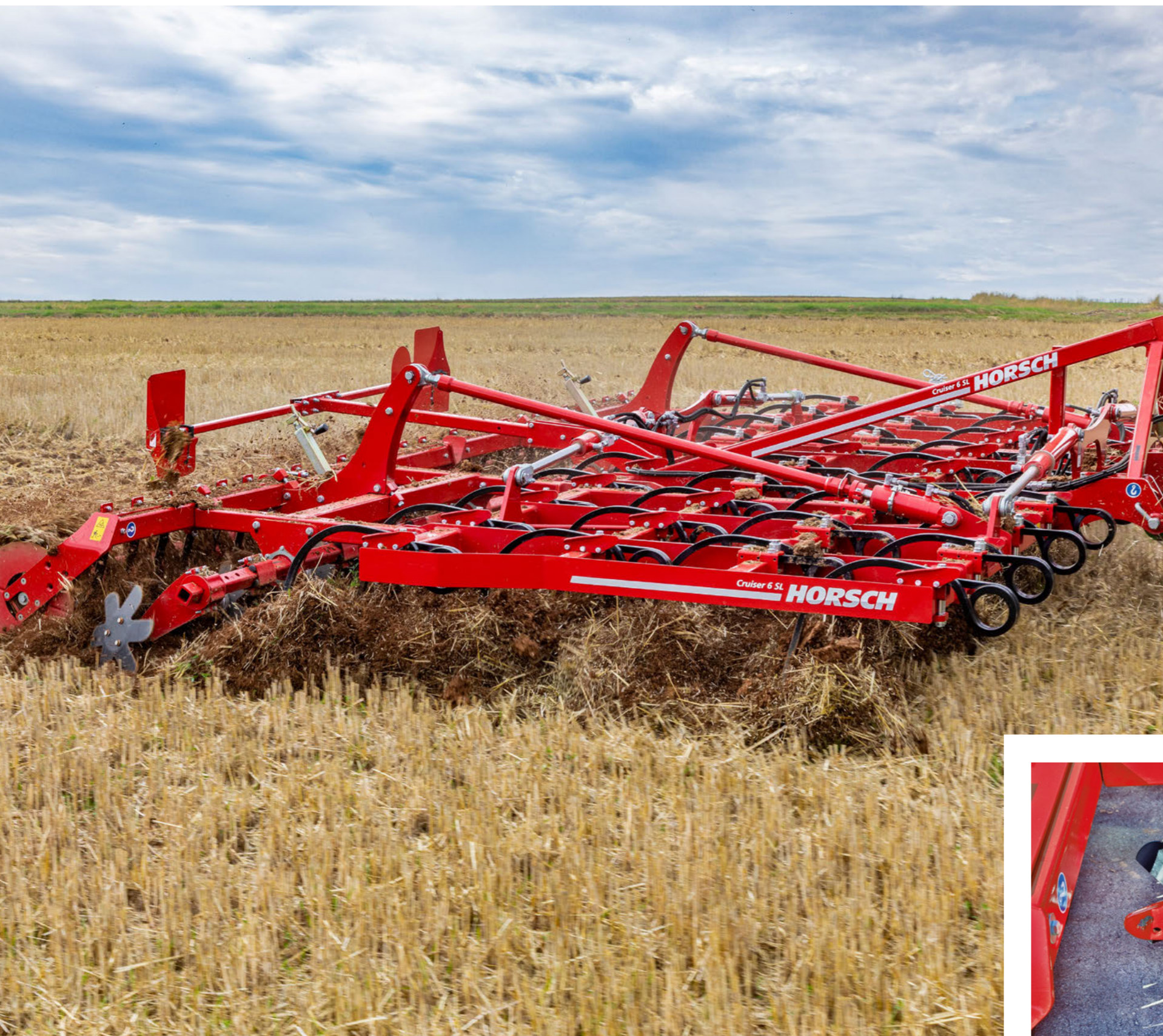
Rubber-cushioned levelling discs to protect from obstructions
