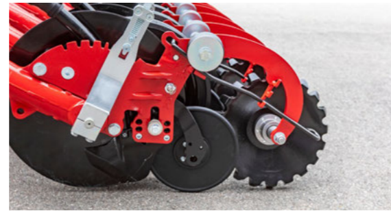
Steel star roller – produces fine soil and closes the seed furrow
