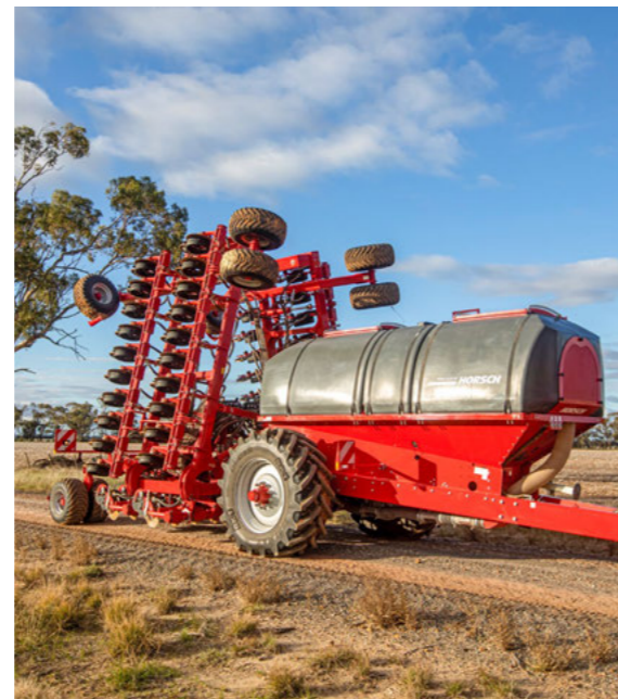
Seed wagon with a capacity of 12 000 l and a 50:50 partition
