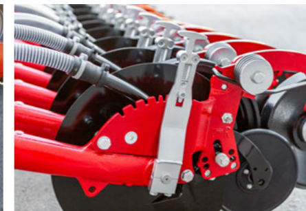
Finely graduated individual depth adjustment without tools
