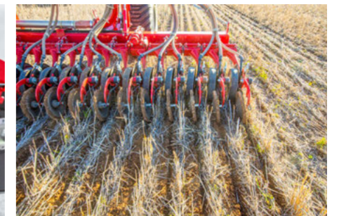
Low disturbance due to SingleDisc seed coulters
