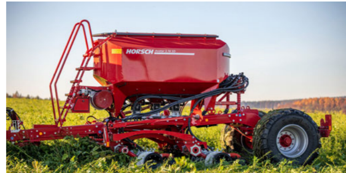
3 800 l double hopper or triple tank
