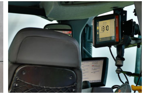
Digital, easily readable display of the filling level in the terminal
