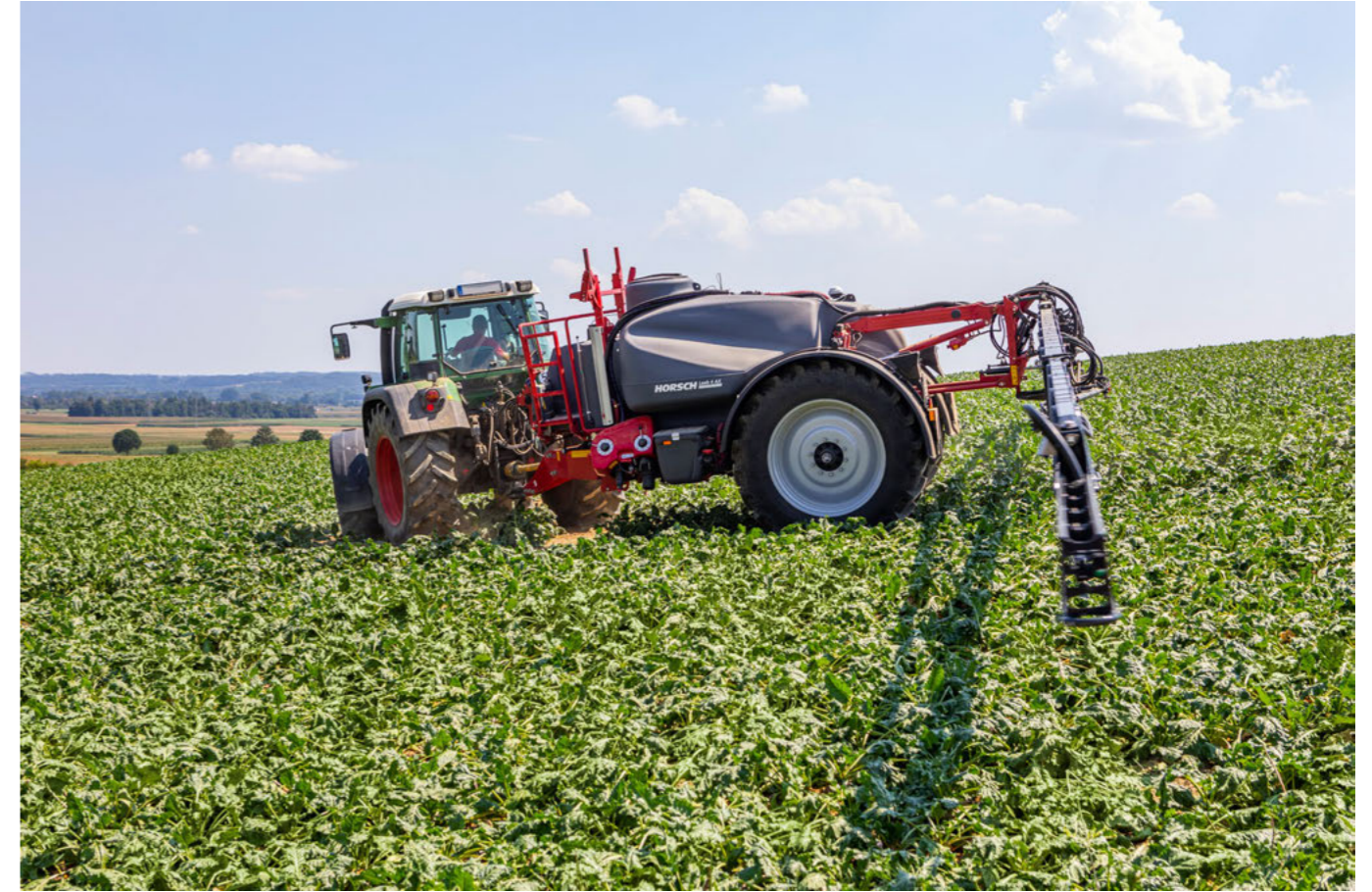
Drawbar steering: crop protection and precise following in the tractor track
