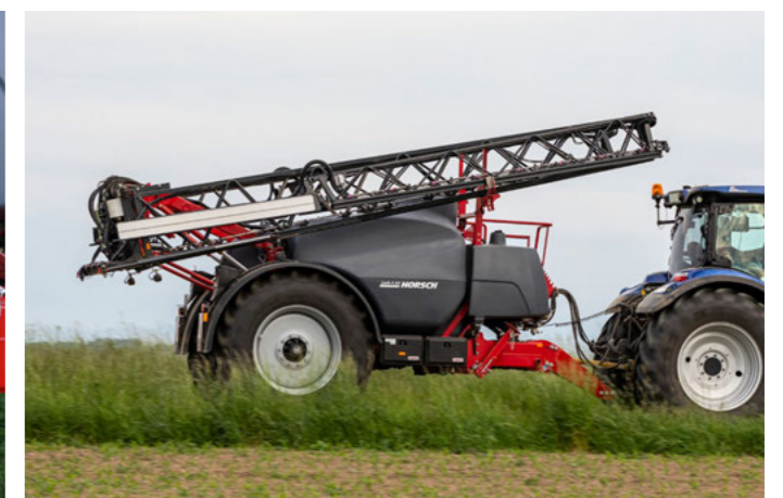
5-part boom with compact folding
