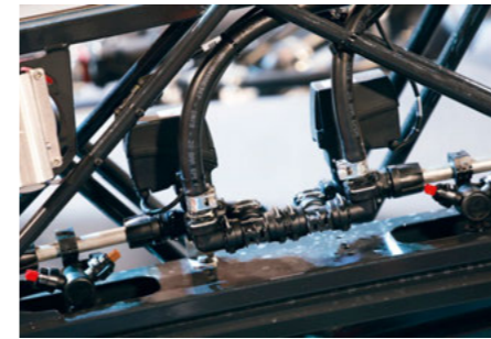
HORSCH Leeb 4 AX – electric nozzle control
