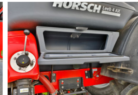
Practical storage compartment directly at the induction hopper as standard
