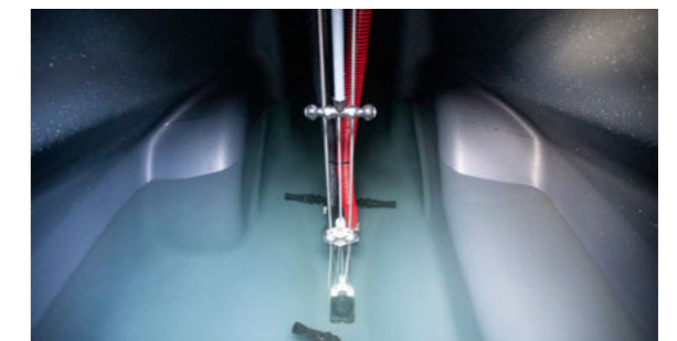
Leeb 4 AX inside view of the tank: powerful agitator and cleaning nozzles
