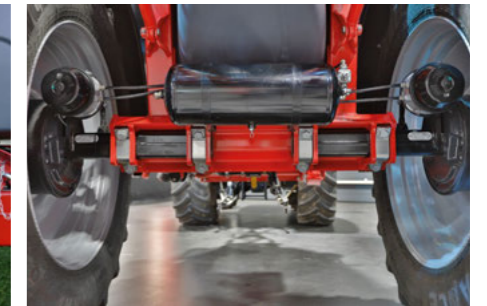
Full-floating axle for mechanical adjustment of the track width from 1.50 to 2.25 m depending on the tyres
