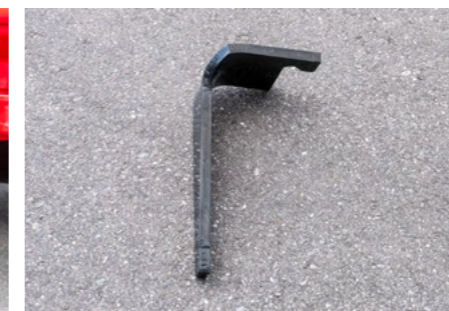
Tines on grip turn the power harrow into a rotary cultivator
