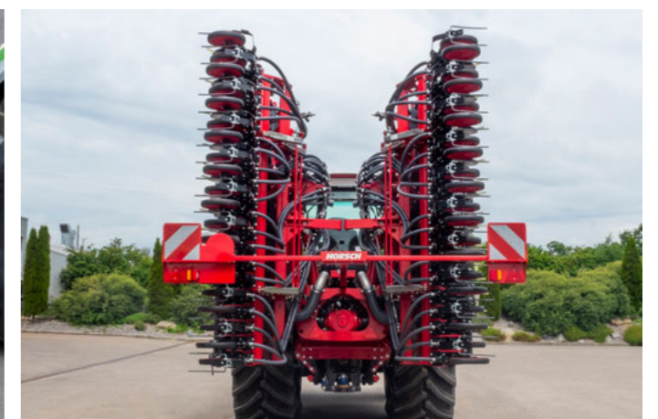
Versa 6 SL in road transport position
