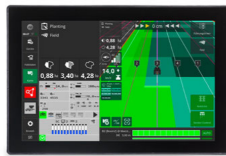
With single grain seeding technology and HORSCH AutoLine, tramlines can be sown completely flexibly and independently of the driving direction supported by GPS.
