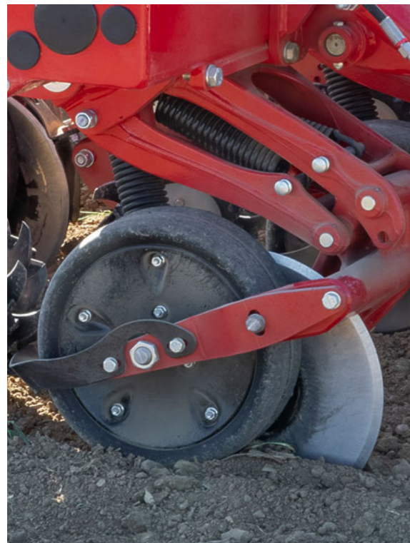
Single disc fertiliser couler
