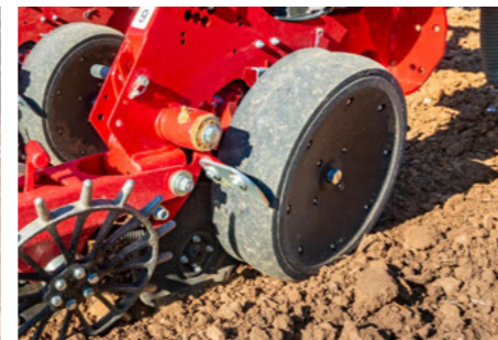
Standard depth control wheel for normal soils
