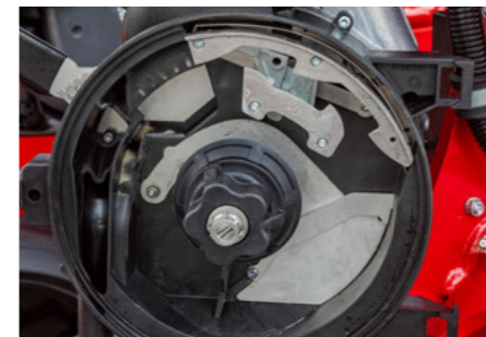
The universal singulator does not have to be adjusted
