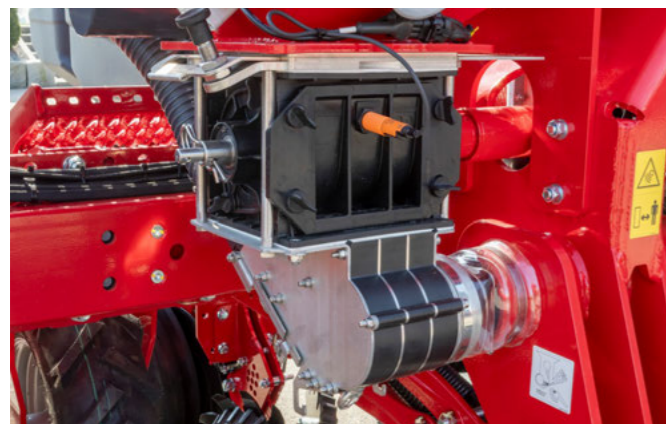
One of the fertiliser metering devices
