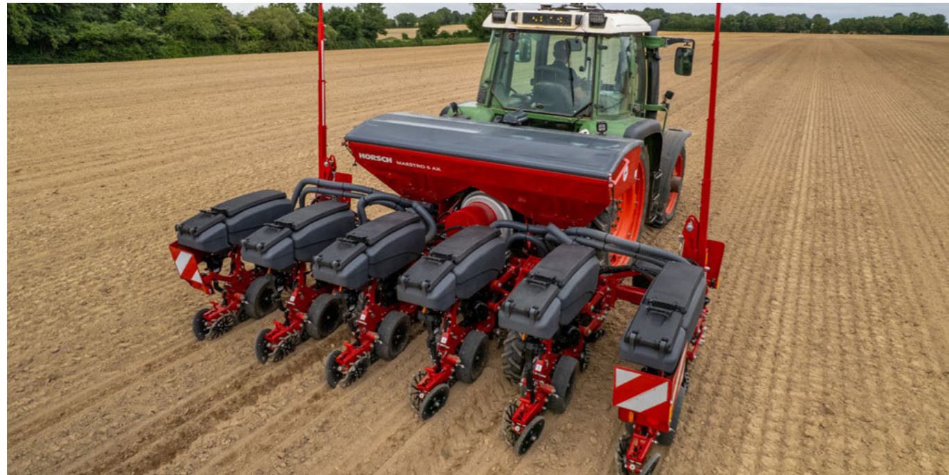
1 100 L fertiliser hopper with half-side control
