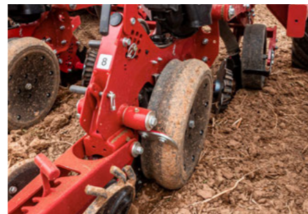
RID wheel reduces soil compaction directly at the seed slot in very hard or direct seeding conditions
