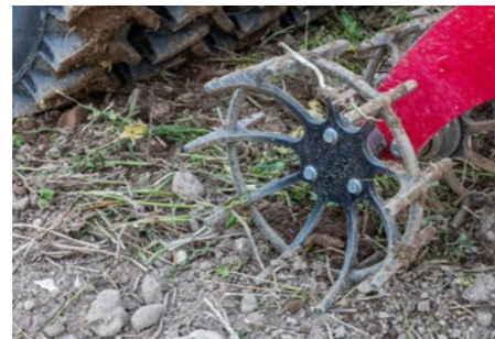
Focus TD crumbling levelling system
