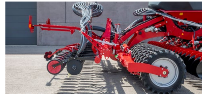
1-row tyre packer for even consolidation
