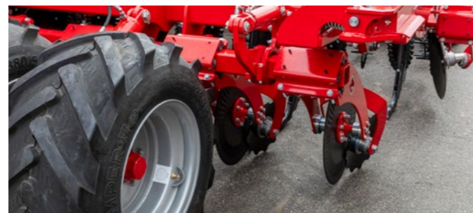
Pre-cutting directly in front of each tine
