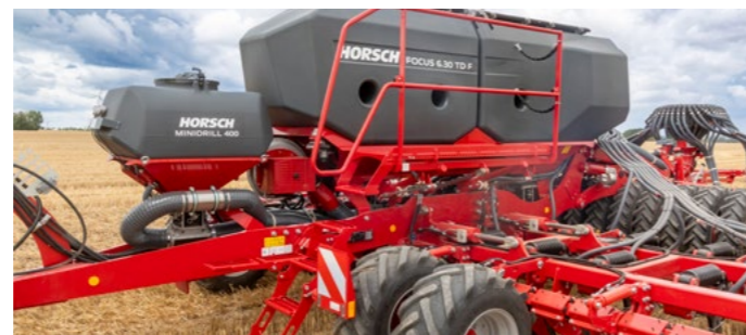
MiniDrill G&F as third component
