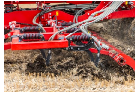
LD point /LD Plus point – mixing of the loosened area
