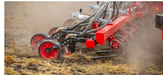
SeedFrame with TurboEdge tine coulters
