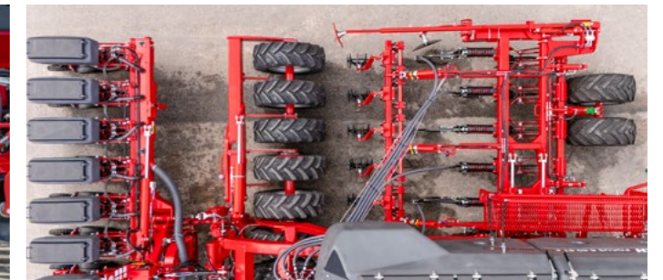
Tyre packer directly behind the loosening tine
