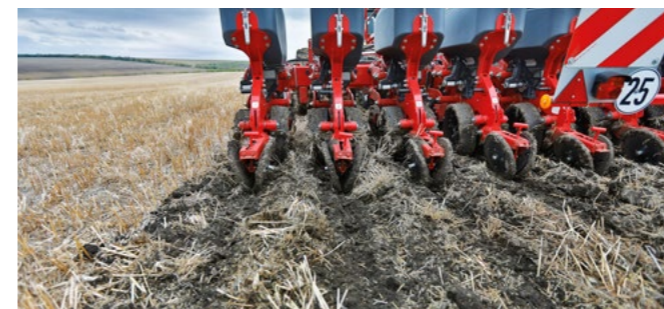
StripTill with singulation
