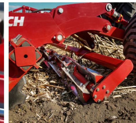
Optional with hydraulically pre-tensioned knife roller for an additional crushing effect.
