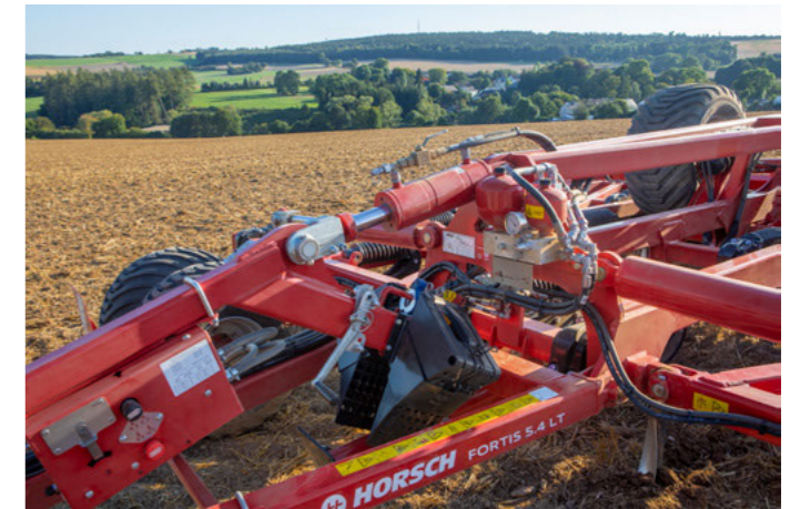
Integrated load transfer to the rear axle of the tractor without any additional coupling points
