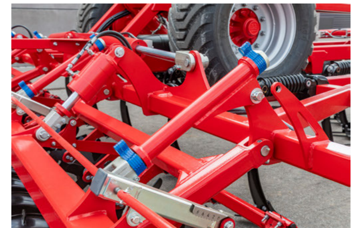
Packer angle adjustment for all double packers to quickly react to changing conditions
