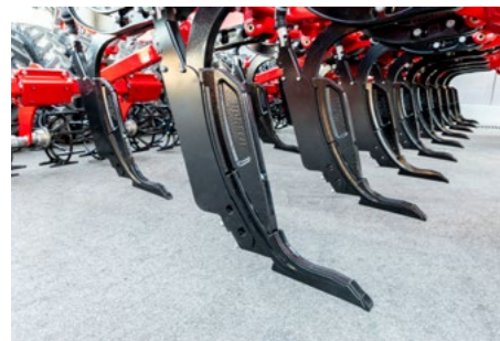
ULD point loosens without mixing
