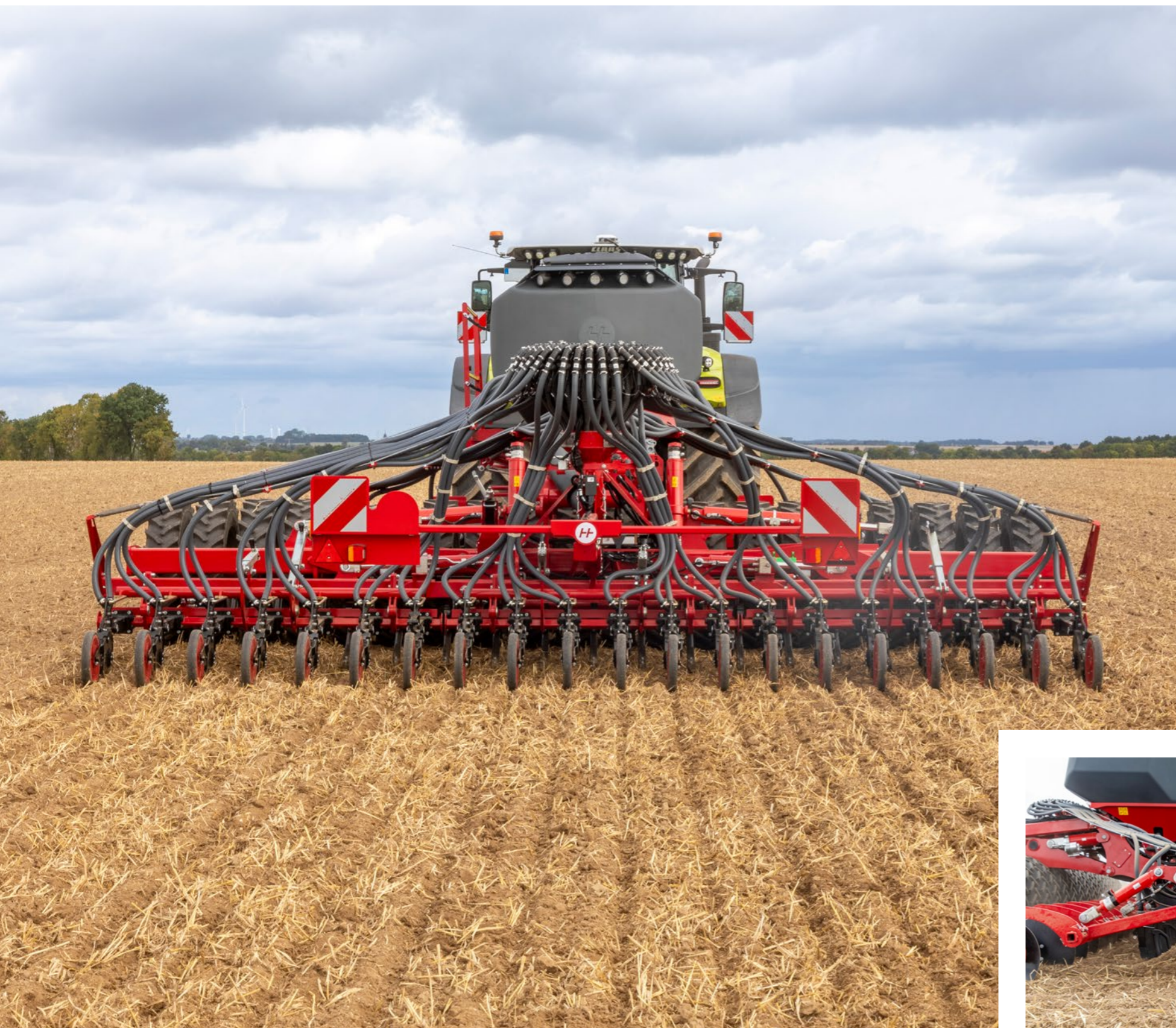
Focus for deep loosening with simultaneous depot fertilisation
