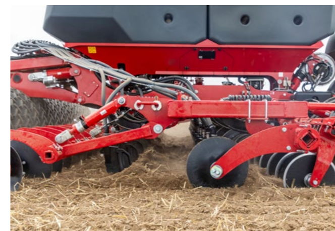
Focus for deep loosening with simultaneous depot fertilisation
