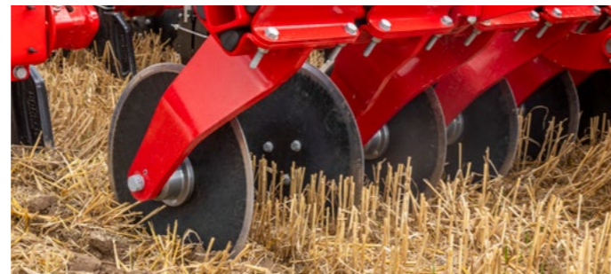
1-bar design directly in front of the tine
