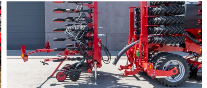
Easy seed bar replacement due to 3-point linkage
