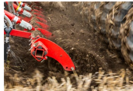
Fine soil production with the crumbling levelling
