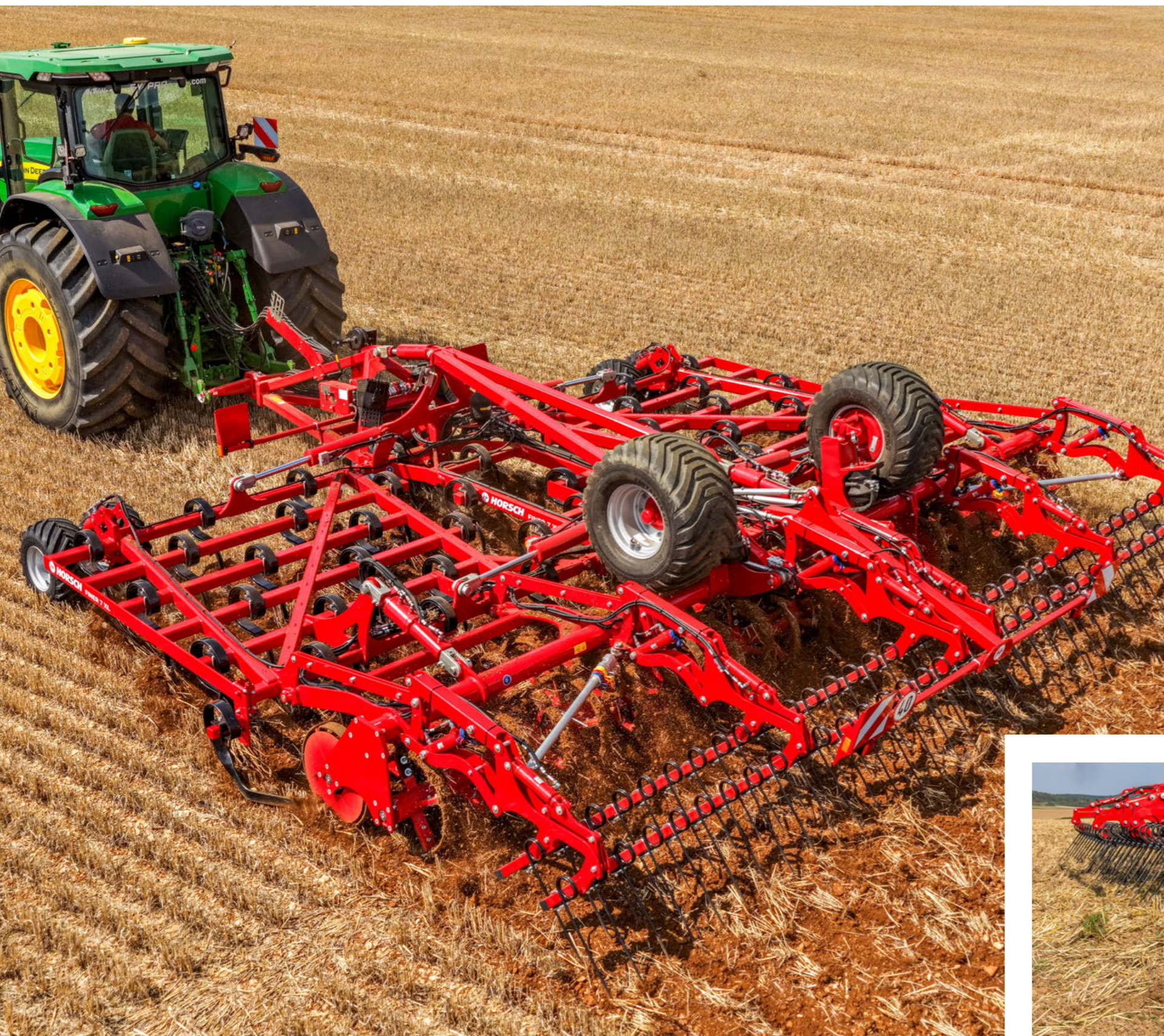
Harrow places uprooted weeds on the surface
