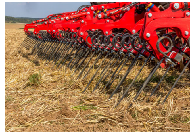
Harrow places uprooted weeds on the surface
