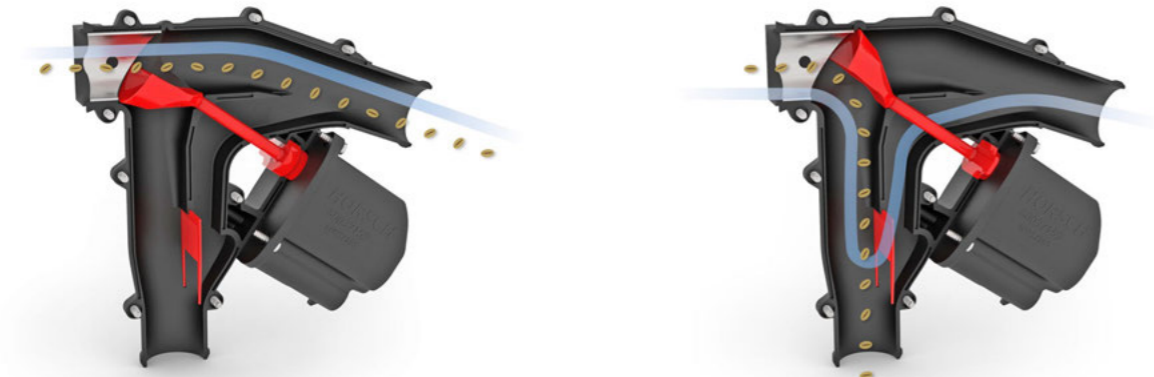
RowControl flap open: seed is transported to the coulters
