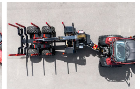
The forwarder can be laterally shifted by up to 104 cm with the drawbar
