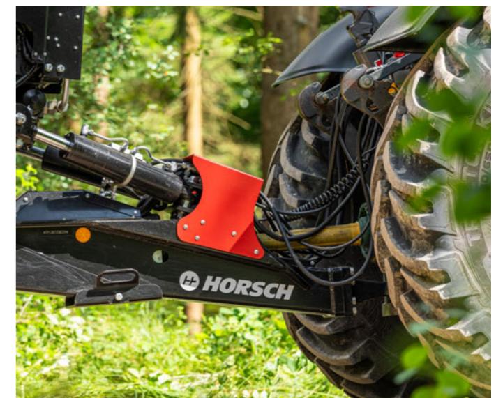
Pto-shaft pump installed in the drawbar for driving the onboard hydraulics
