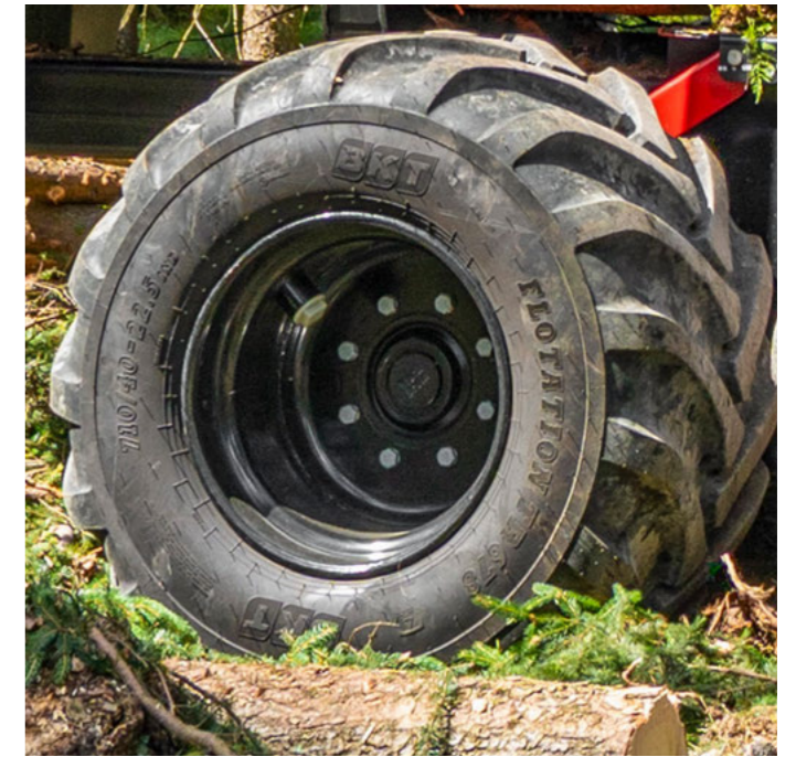
BlackBruin wheel drive on the rear axle of a Pirk 20 MP forwarder trailer
