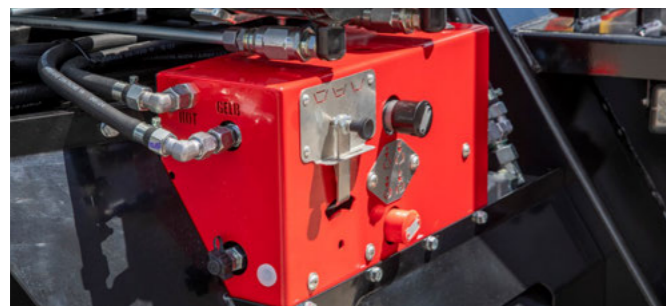
Brake load adjustment at the drawbar
