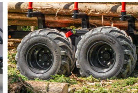
Tyres up to 710 mm wide and a diameter of 117 cm
