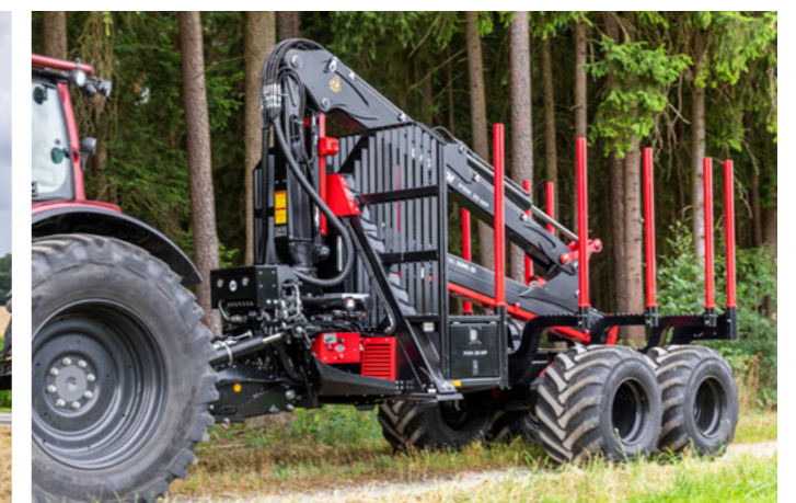
On field and forest tracks, the wagon is lifted via the hydraulic drawbar for more clearance.
