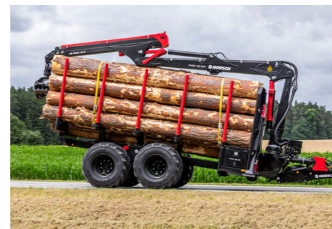
By lowering to the end stop, the drawbar is secured against lateral movement.
