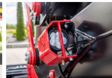
WorkLight: protected crane headlight as an option
