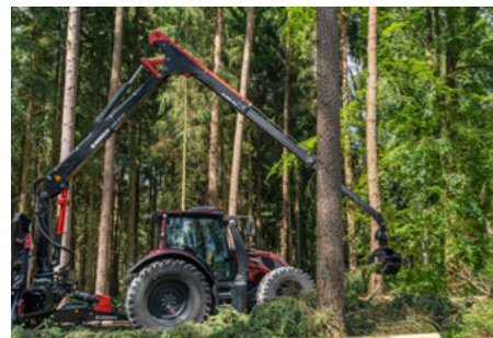
Swivel range up to 400° also allows for working in front of or next to the tractor
