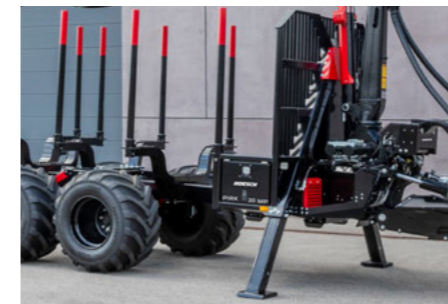
A-column support integrated into the front grid
