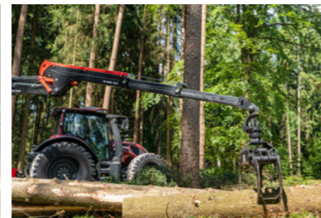
All cranes are equipped with a double telescopic extension.
