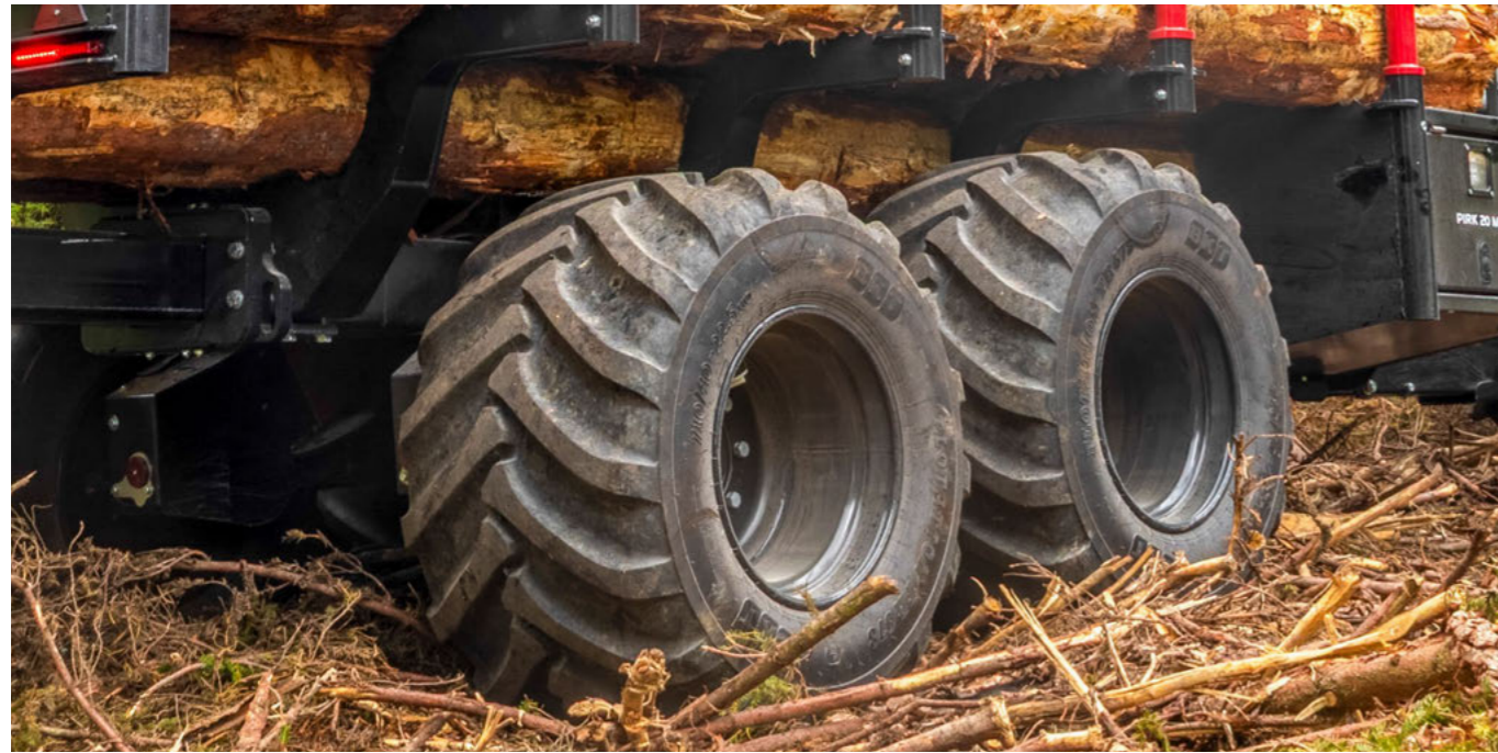
Bogie transport wheels with a swivel range of up to \pm 20^\circ
