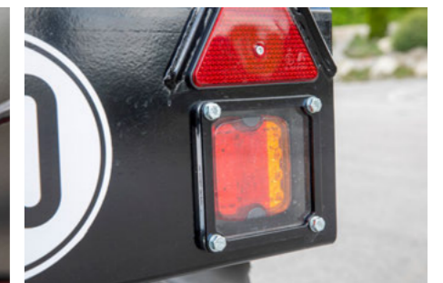
Protected installed lighting system
