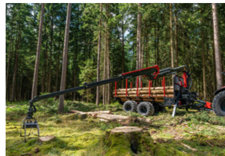
IB 9800.L10 with up to 10 m range and 2.2 t lifting power with an outreach of 4 m
