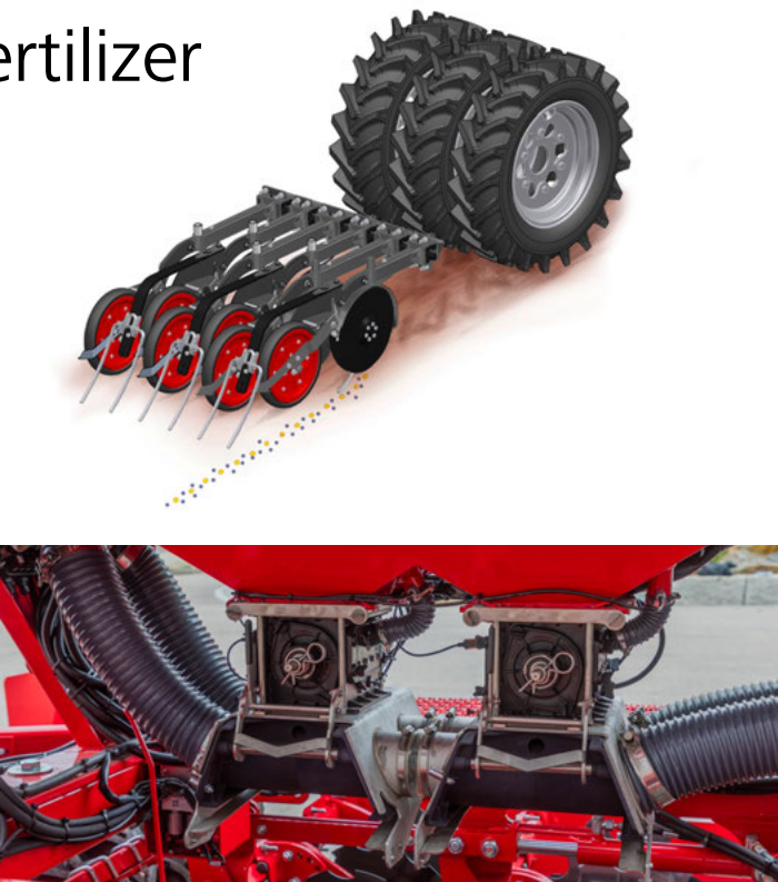
Double hopper S&F – meter different components separately and place them together in the furrow
