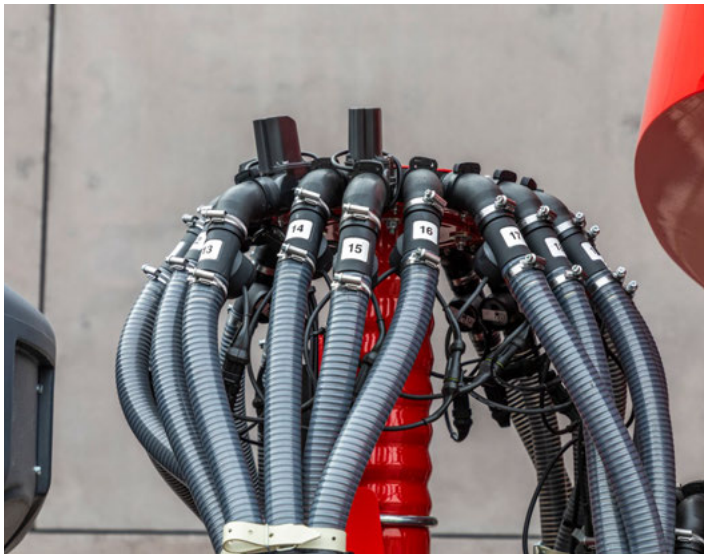
Fertilizer and seed flow control – for a permanent monitoring of the seed and fertilizer hoses
