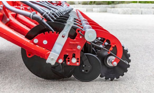
Steel star roller – produces fine soil and closes the seed furrow
