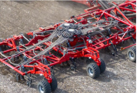
Big support wheels for precise seeding depth
