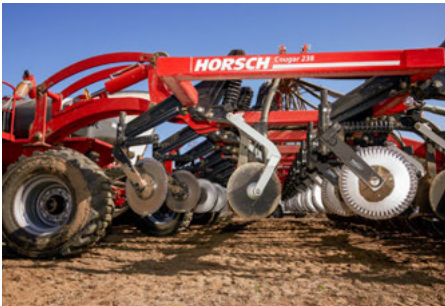
Unique 2-rank design provides narrow contour depth for precise seed placement in extreme variable field terrains
