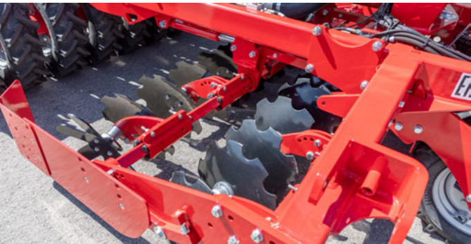
DiscSystem Pronto with attachment frame for track eradicator discs
