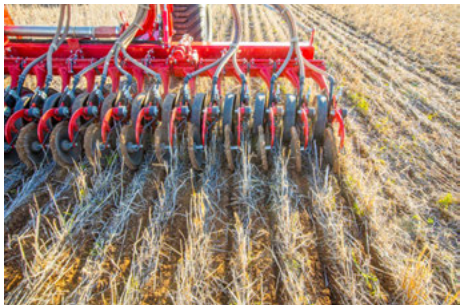
Low disturbance due to SingleDisc opener
