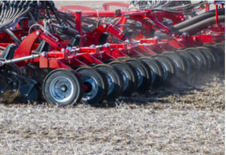
Packer wheels for excellent seed to soil contact
