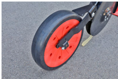
3" wide press wheel – ideal on light soils
