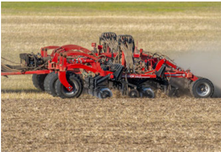
Smooth and directed hose routings ensure consistent flow of product at each opener.
