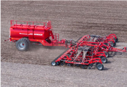
Panther with 4-ranks for optimal flow of residue
