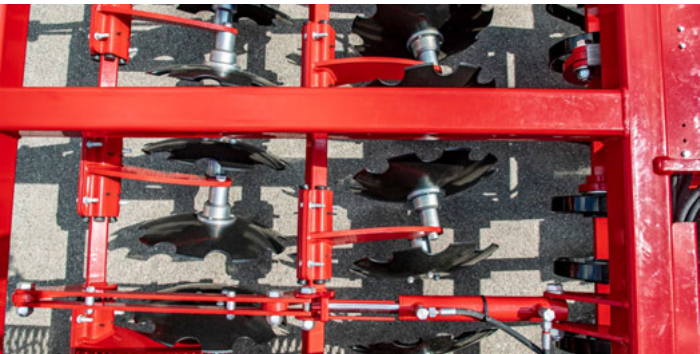
DiscSystem Pronto – 18” disc with serrated profile
