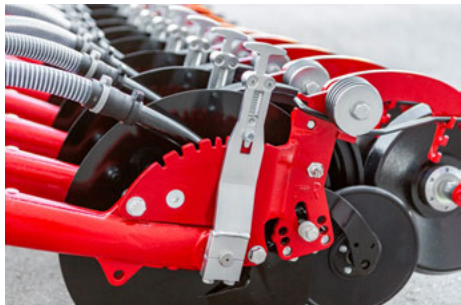
Finely graduated individual depth adjustment without tools
