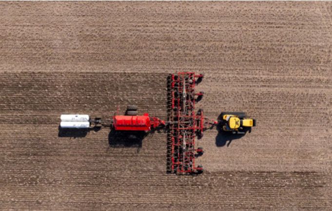
SW 600 as a tow-between cart with extra hitch for anhydrous cart
