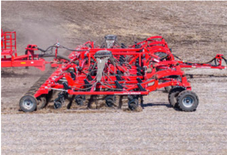
4-ranks of shanks and 15 inch shank spacing for no-till seeding
