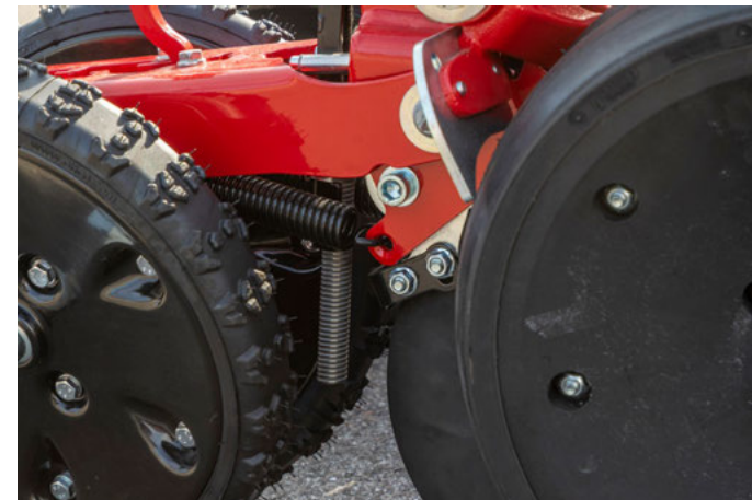
Liquid fertilizer application behind the catching roller
