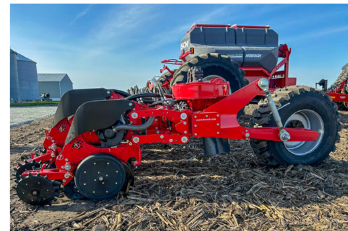
Standard RowUnit with proven AirVac singulation
