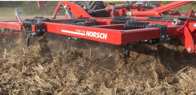
4-bar design for intensive mixing
