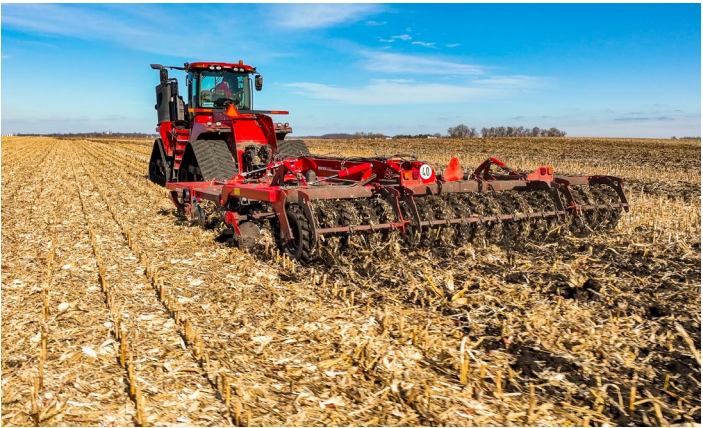
Intensive tillage due to discs and shanks
