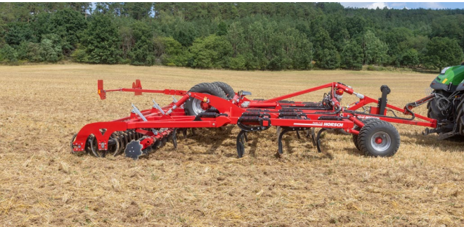
Rigid packer frame with double packer
