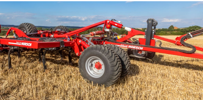
Front support wheels for even depth control
