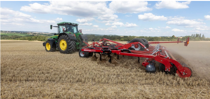
Steelflex packer with hydraulically pre-tensioned RingFlex
