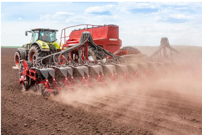
Hydraulic coulter pressure up to 350 kg for reliable seeding even in heavy conditions
