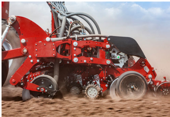
Wide parallelogram with large bushings for good stability and long durability
