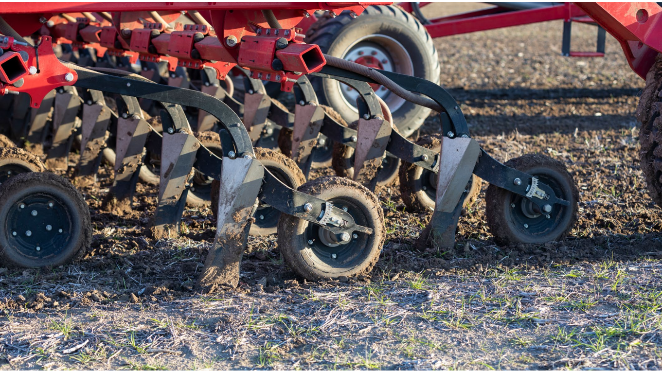
Perfect seed placement due to individual depth control
