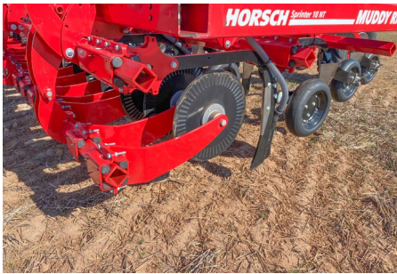
Sprinter NT tine with individual depth control
