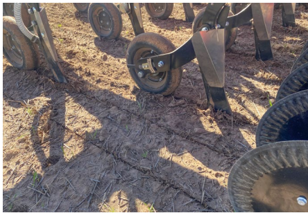
Minimum movement of the soil due to cutting disc and narrow tine
