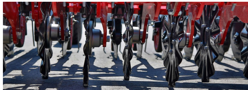
Ondulated disc 13x undulated Ø 18 – 30 mm wide – recommended on light soils
