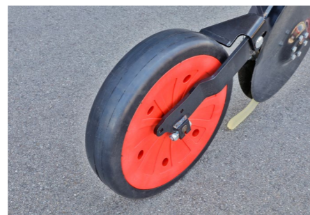
7 cm wide press wheel – ideal on light soils
