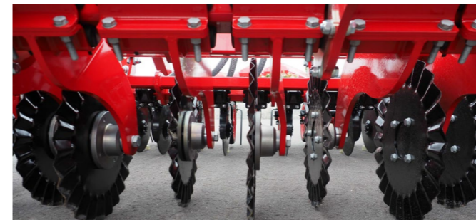
Loosening of the surface and production of enough fine soil for an optimum embedding of the seed
