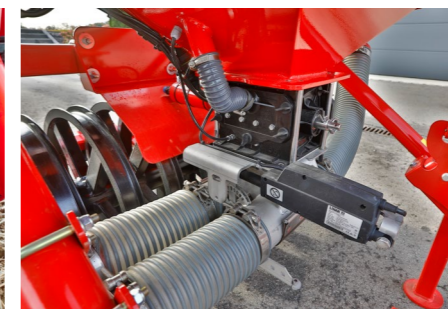
The electric half-width shut-off can be automated with a SectionControl activation.
