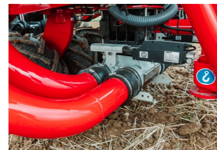
Electric half-width shut-off – switching the half-width on and off easily via a button in the terminal
