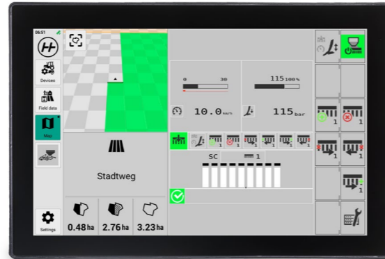
By displaying up to 3 widgets in addition to the main workin screen, the user can keep track of several applications at the same time.
