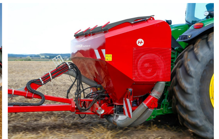
Double hopper with a capacity of 2 800 l
