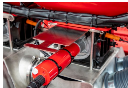
Pressurised hopper system with open valve
