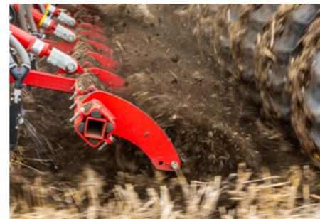
Fine soil production with the crumbling levelling
