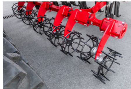
Focus 3 TD with crumbling levelling
