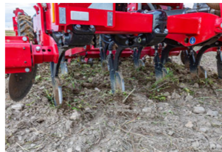
ULD point opens the soil and places fertiliser
