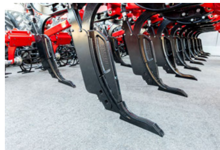
ULD point loosens without mixing
