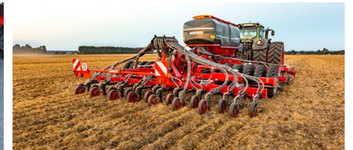
TurboEdge seed coulters for sowing in soils with a lot of straw
