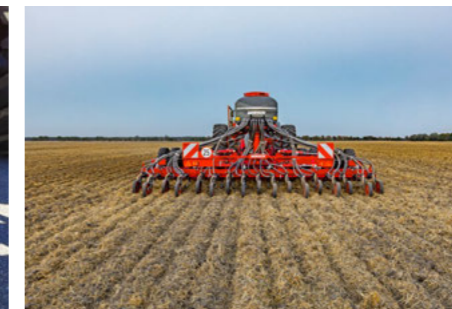
Residue free seed furrow due to TurboEdge tine seed coulters
