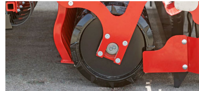
Trapeze ring packer 50 cm diameter
