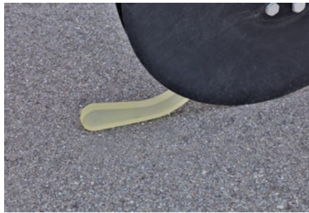
The HORSCH Uniformer ensures a precise fixing of the seed
