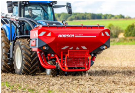
Partner 2000 FT with 60:40 partition allows for applying seed and fertiliser, 2 x seed or two different fertilisers
