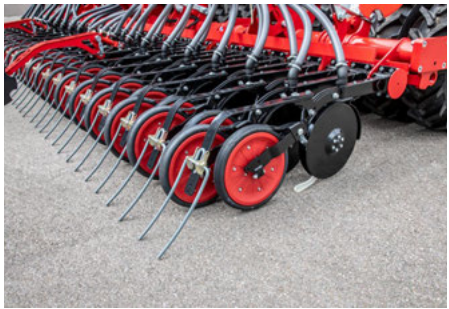
HORSCH TurboDisc seed coulters
