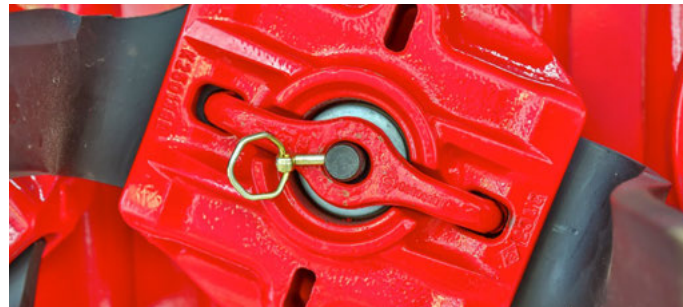
Tines can be changed without any tools
