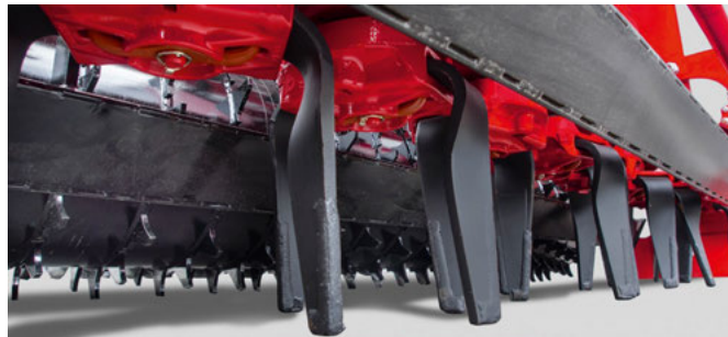
Deflector rail in the front is available as an option
