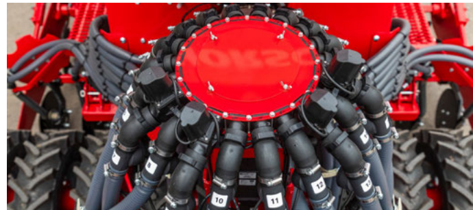
Monitoring of the pneumatic flow at the distribution tower
