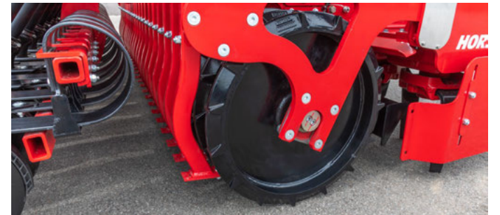
Trapeze ring packer 60 cm diameter
