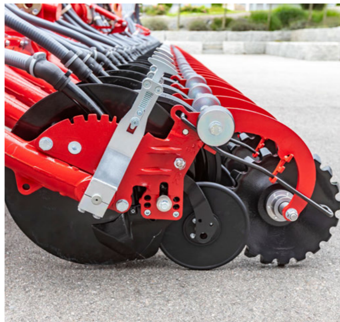
Steel star roller – produces fine soil and closes the seed furrow
