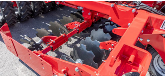
DiscSystem Pronto DC with attachment frame for track eradicator discs
