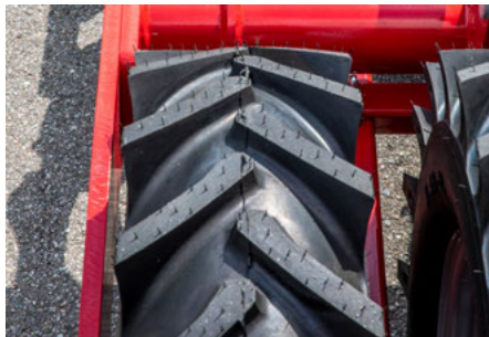
Straight tyre profile increases consolidation in the consolidation area
