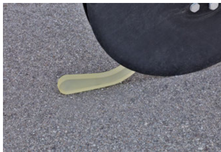
The HORSCH Uniformer – TurboDisc seed coulters ensures a precise fixing of the seed
