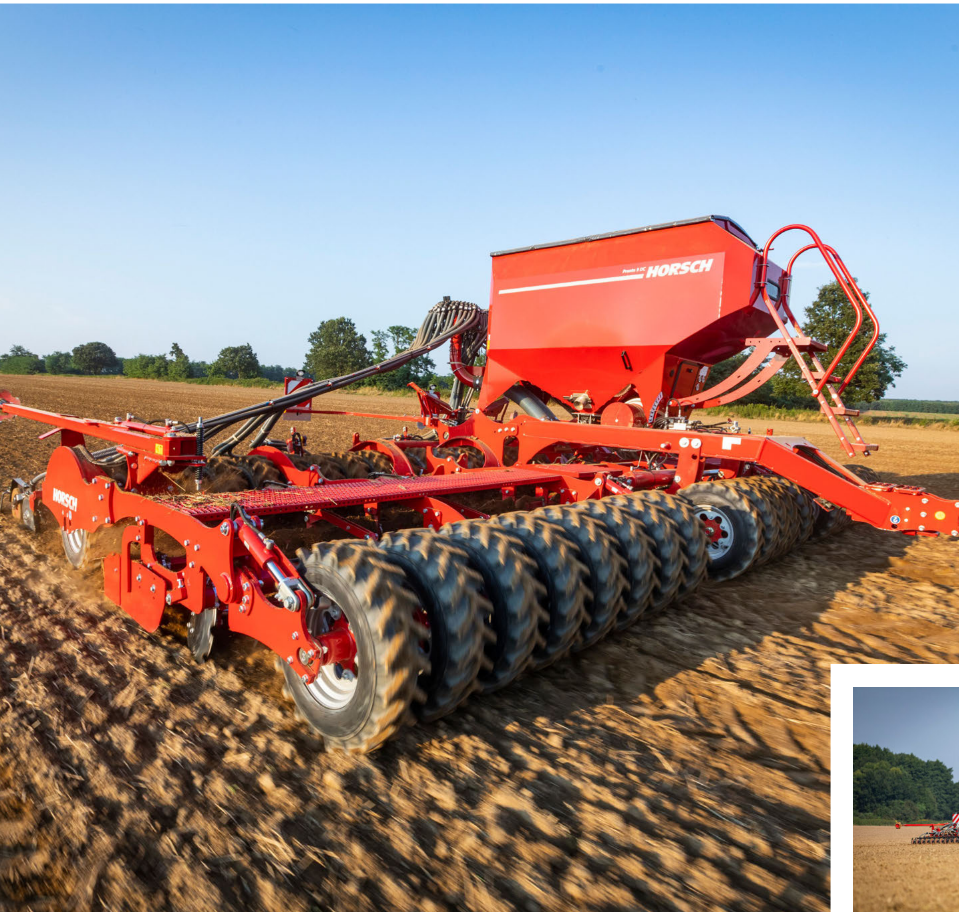
The TurboDisc seed coulters have been designed for a precise seed placement at high operational speeds
