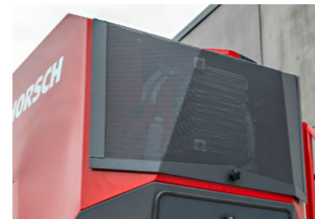
Oil cooling on the hydraulic fan – heats the air flow in the pneumatic system
