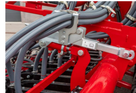
The coulters pressure can be increased via the tractor control device
