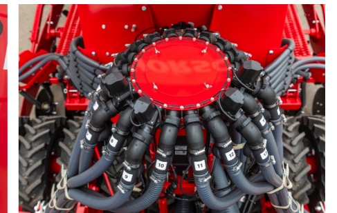
Monitoring of the pneumatic flow at the distribution tower
