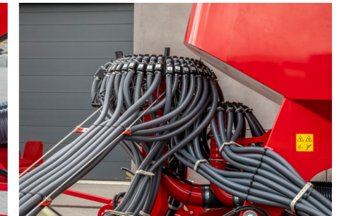
External position of the PPF distribution tower for optimum accessibility
