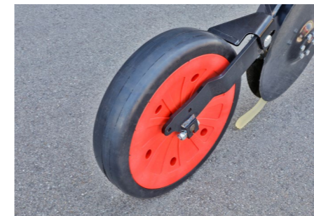
ParaDisc seed coulters – 7 cm wide press wheel
