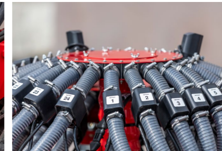
Spelt pneumatics for husk-bearing seeds
