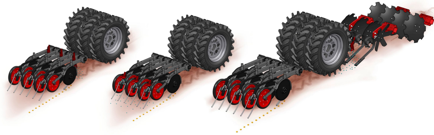
MiniDrill option 9: application via the baffles at the optional Crossbar. Ideal for applying underseeds as they are consolidated again by the tyre packer.
