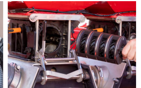
Fine metering insert – rotor
