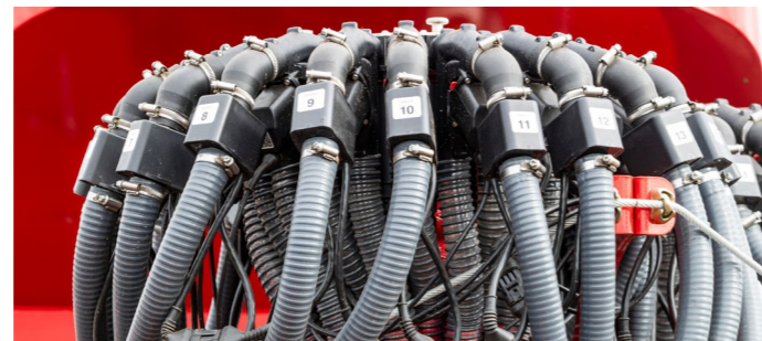
RowControl distribution tower
