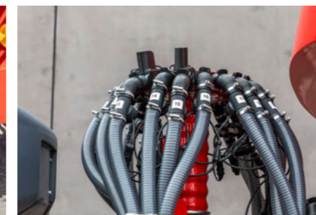
Fertiliser and seed flow control – for a permanent monitoring of the seed and fertiliser hoses
