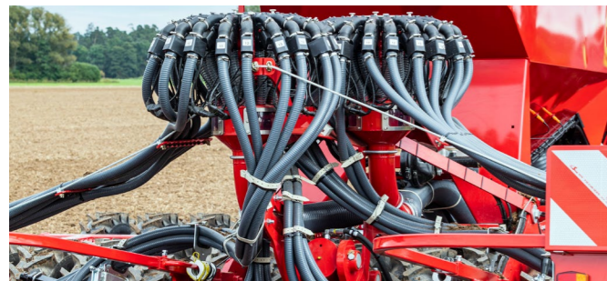
RowControl distribution tower – 2-tower version at the Pronto 6 & 7 DC
