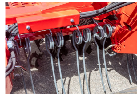
The harrow is placed between the DiscSystem and the tyre packer. The adjustment is carried out mechanically via a hole pattern.
