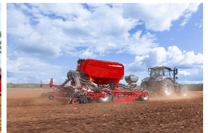
The double hopper system PPF allows for a separate metering and placing of 2 components in 2 horizons
