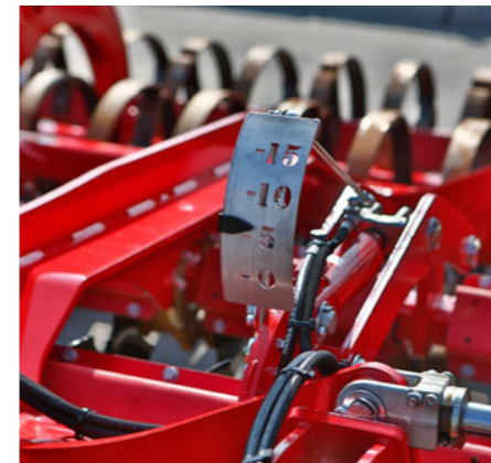
Hydraulic depth adjustment for the comfortable adjustment of the machine
