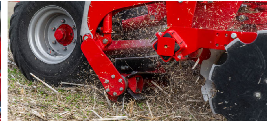
Straw is swirled up by the knife roller
