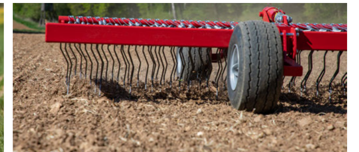
Support wheels are mounted behind each other in one track to run in the same track for example in row crops
