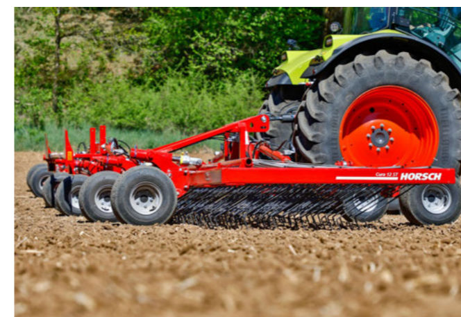
Due to the support wheels, the frame adapts to the contours of the fields
