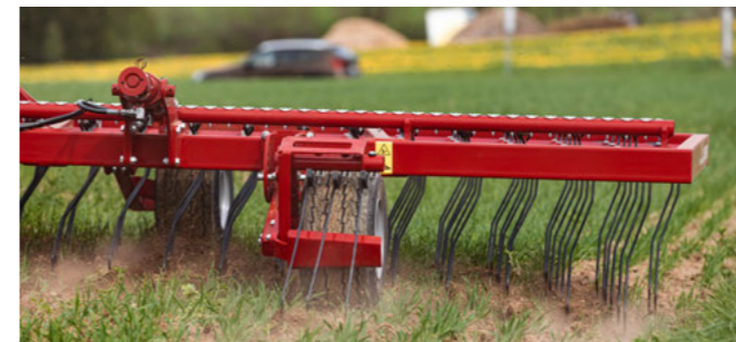
Support wheels are mounted in an offset way to make sure that the crop is not run over twice
